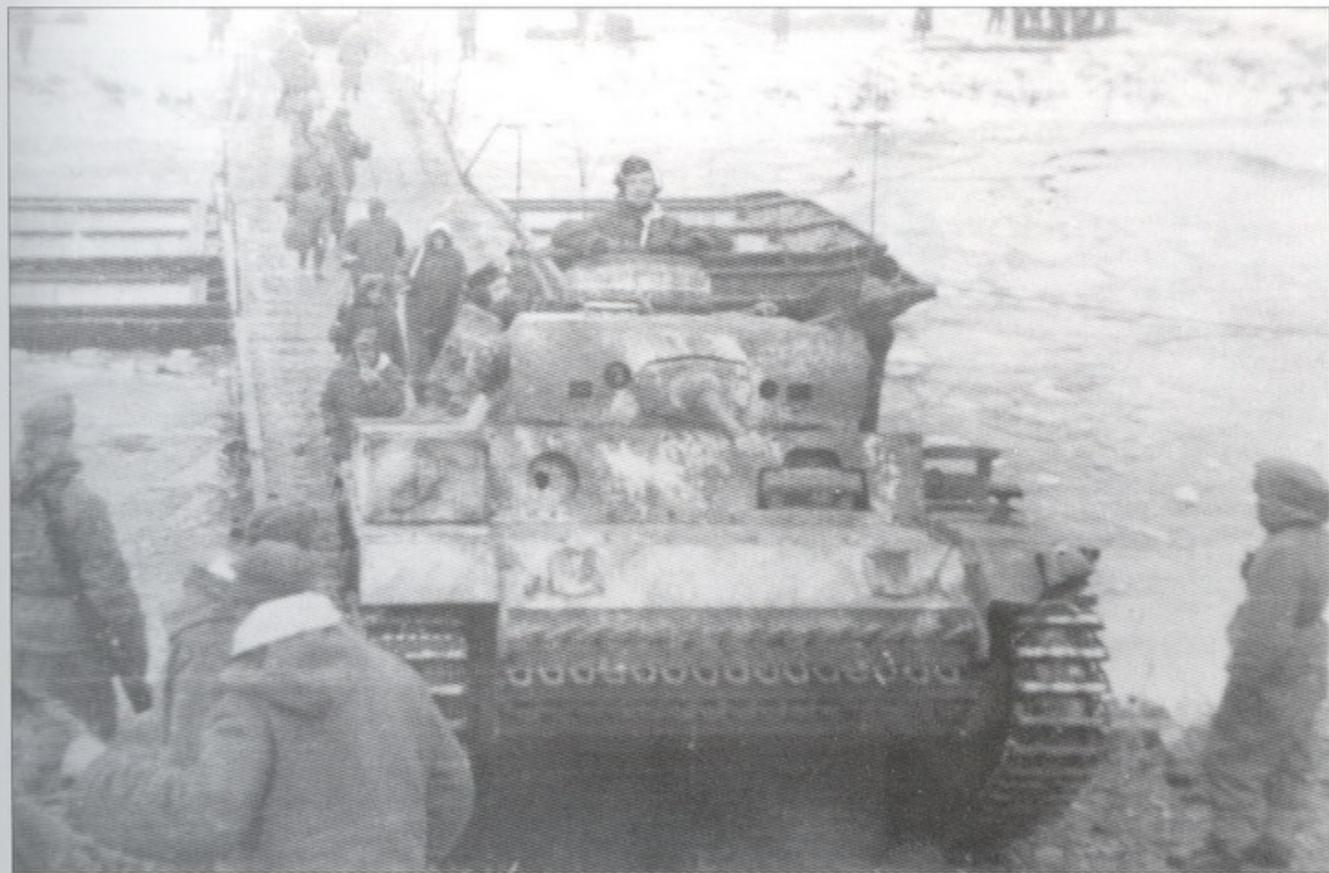
A Pz.Kpfw.III Ausf.L of SS Panzergrenadier Division "Wiking" on the Eastern Front. The Sternantenne D mounted on it indicates that the tank is being employed as a Befehlswagen .
