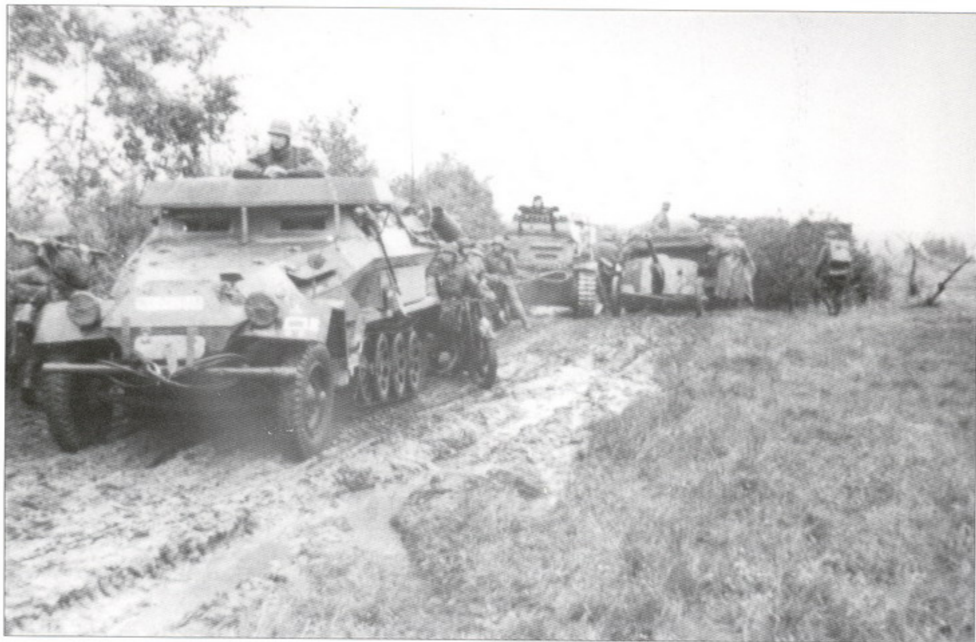
An Sd.Kfz.251/18 Ausf.A ( mittlerer Beobachtungspanzerwagen ) of 1.Panzer Division . It has the characteristic covered table for maps and documents.
