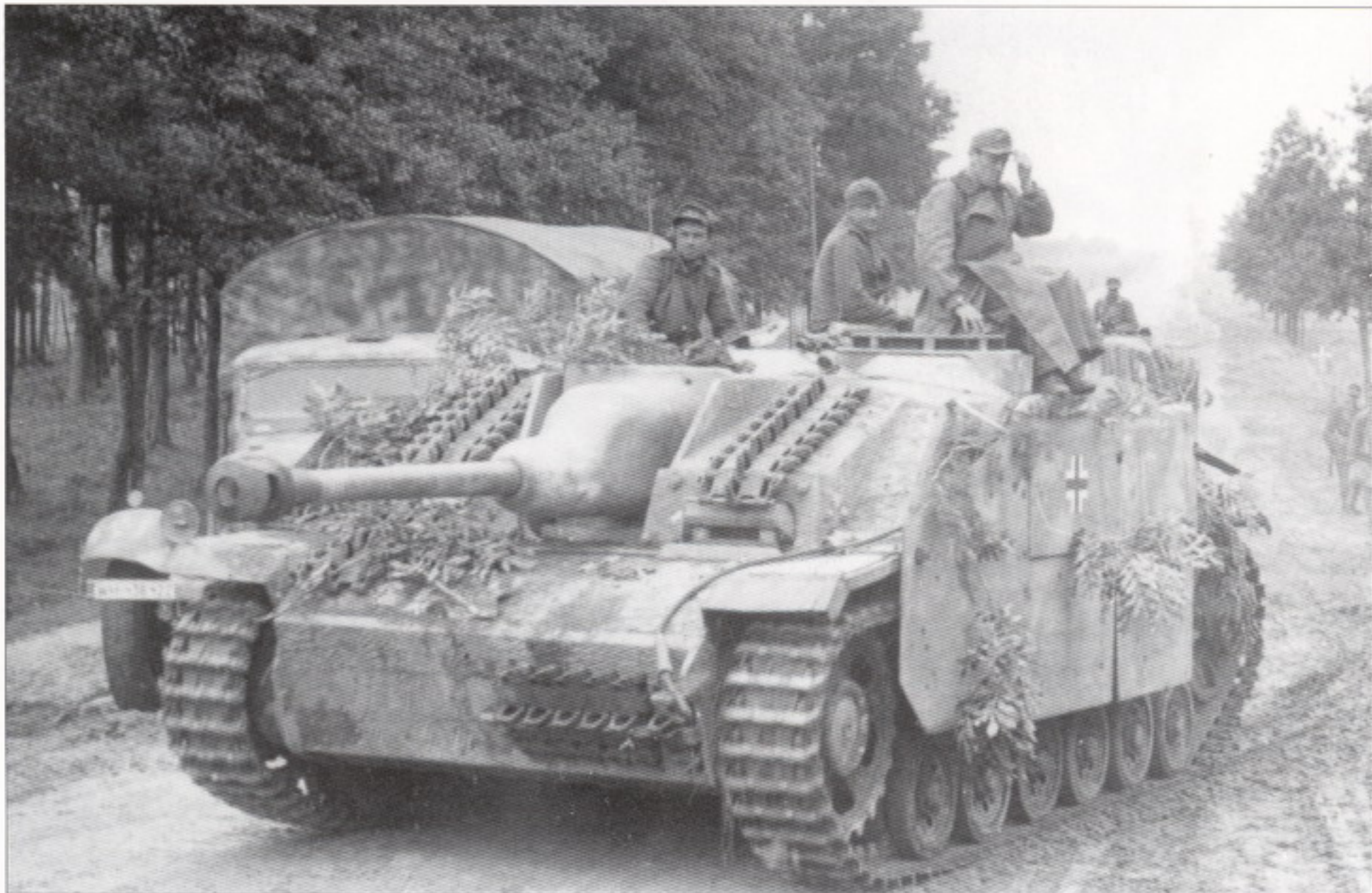
Sturmgeschütze.III Ausf.Gs of 2./Sturmgeschütz.Abt.237 on the Eastern Front 1944. Both vehicles have the Saukopfblende mantlet and the commander's cupolas with additional frontal protection.
