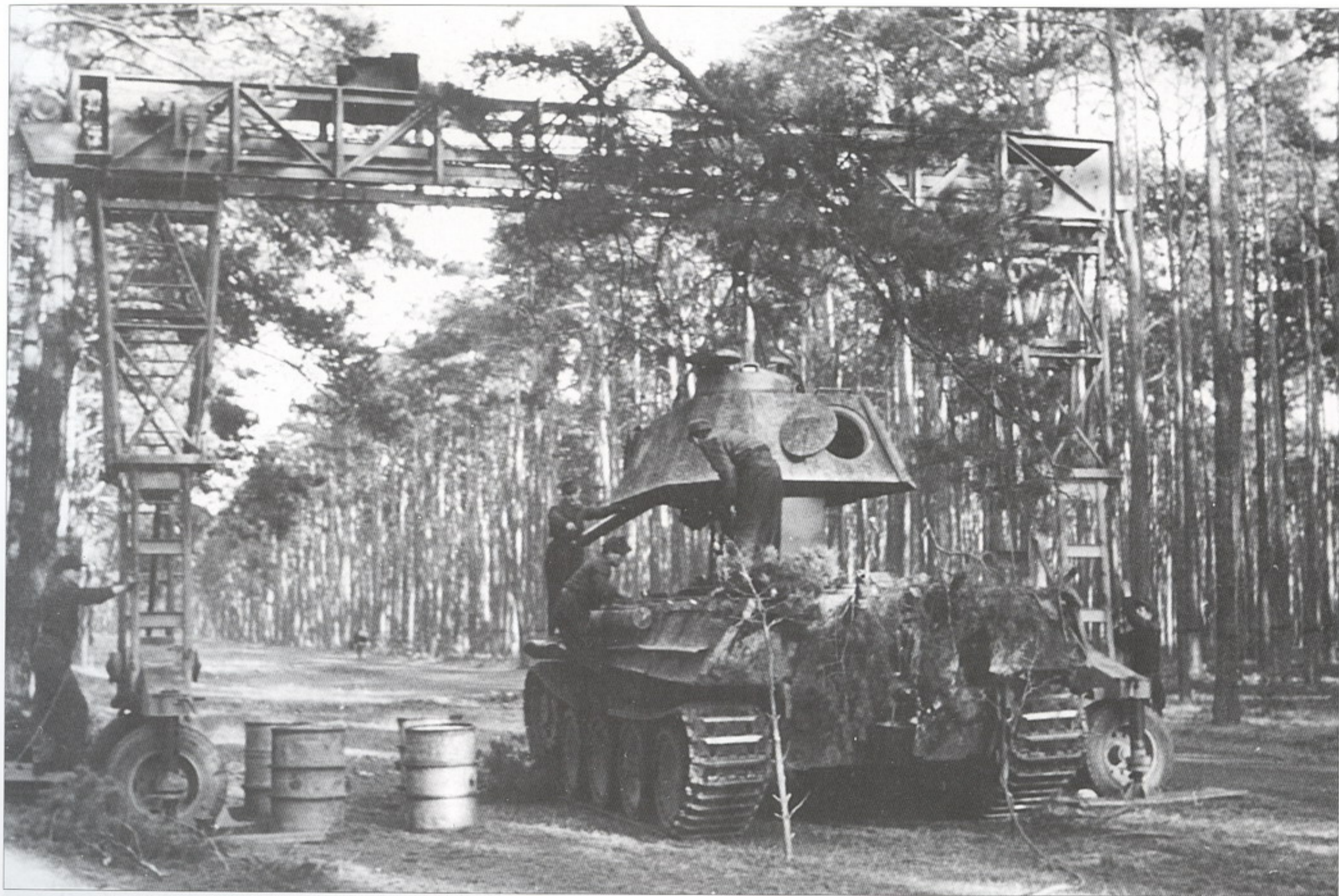
↓ A Panther Ausf.G of Panzer Regiment "Großdeutschland" during repairs, probably in 1945. The 16-ton "Fries" crane is being used.
