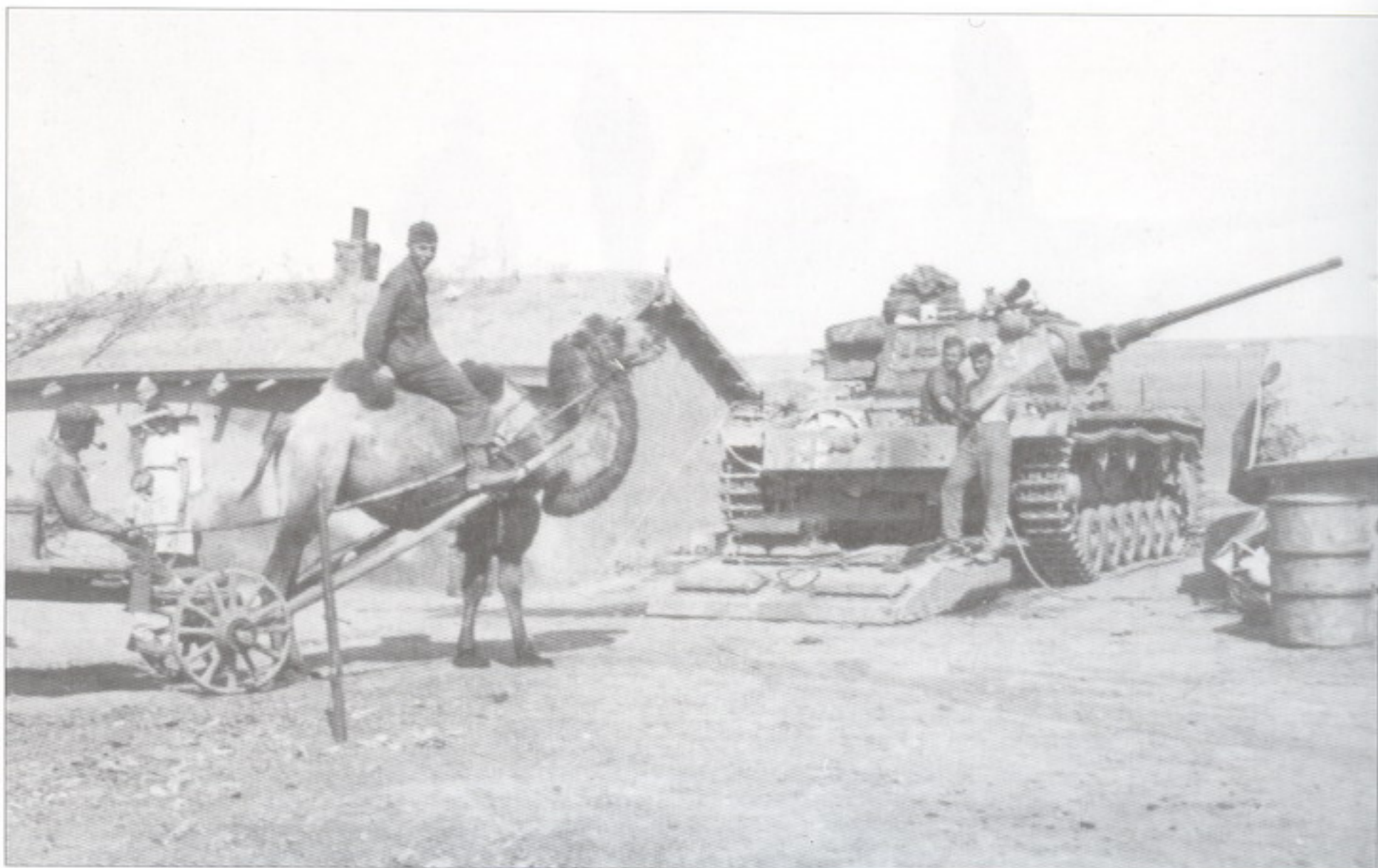
A Pz.Kpfw.III Ausf.L on the southern part of the Eastern Front during an engine change. The entire engine cover has been removed and lies behind the tank.
