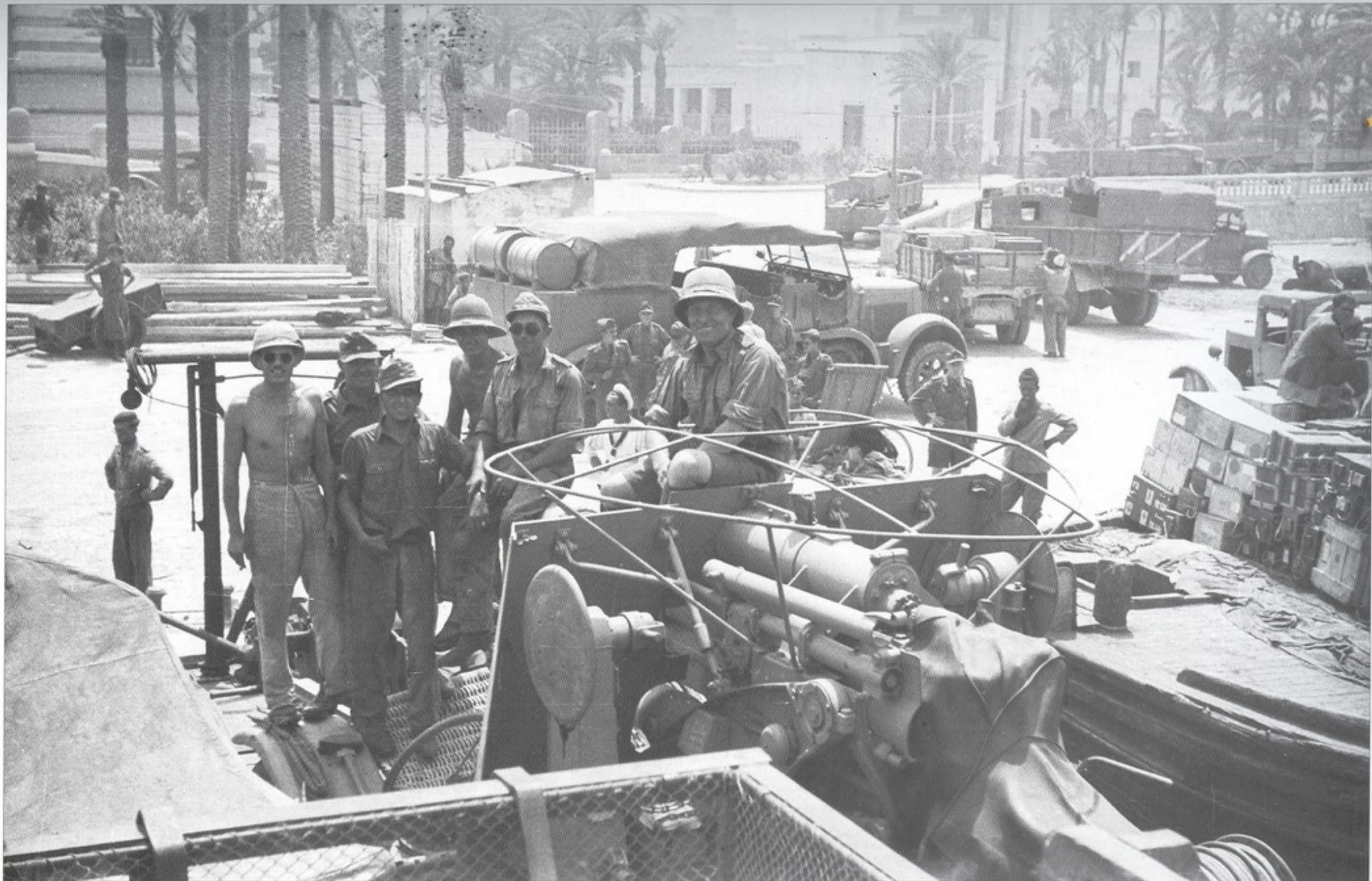
An 8.8 cm Flak 18, with an Sd.Kfz.7 in the background. This halftrack was commonly used to tow the 8.8 gun. The two barrels fastened on the rear of the superstructure are most probably filled with extra fuel.
