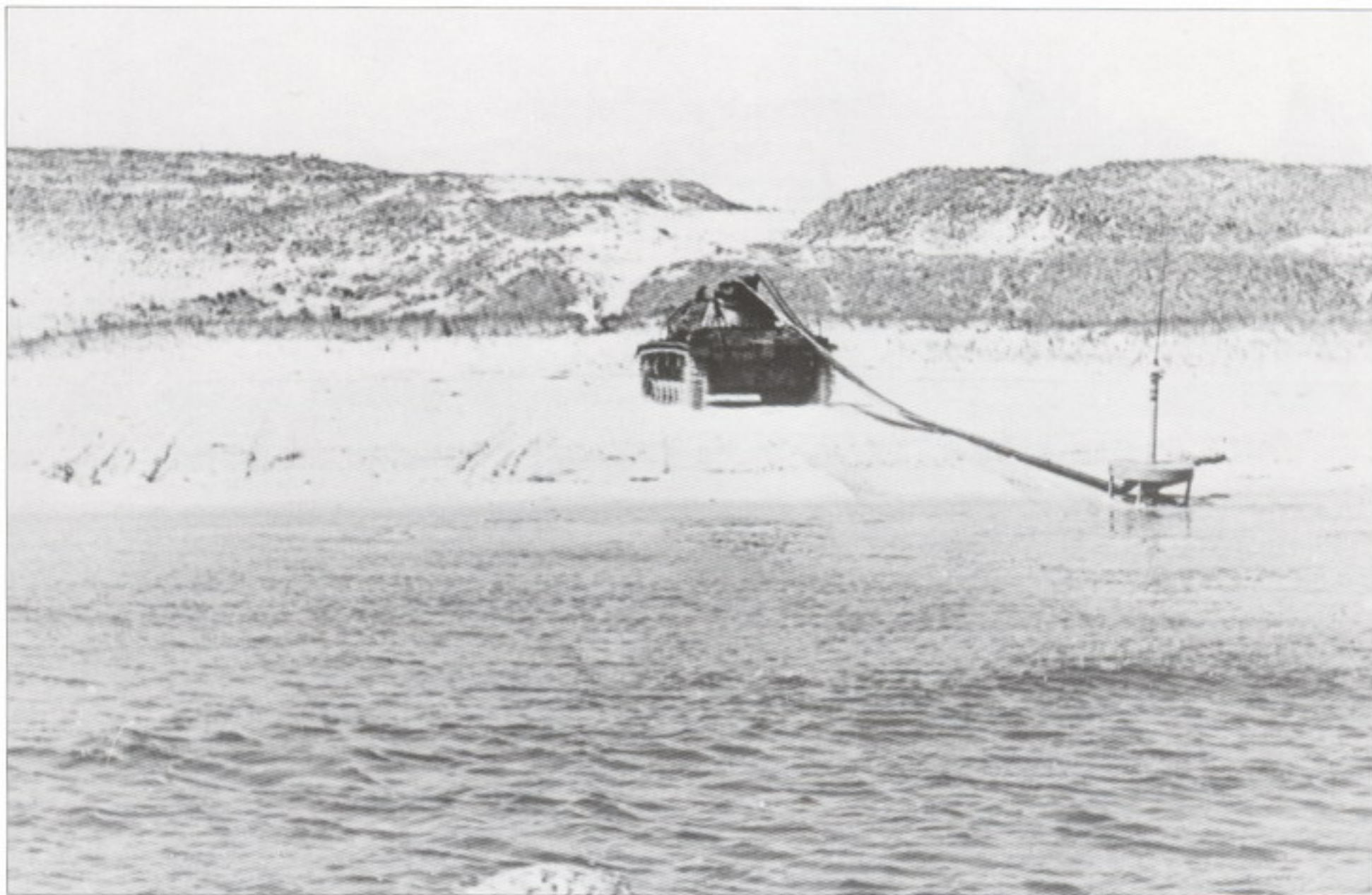
Pz.Kpfw.III Ausf.F (Tauchpanzer) during training for Operation Sea Lion near the island of Sylt in the autumn of 1940.
