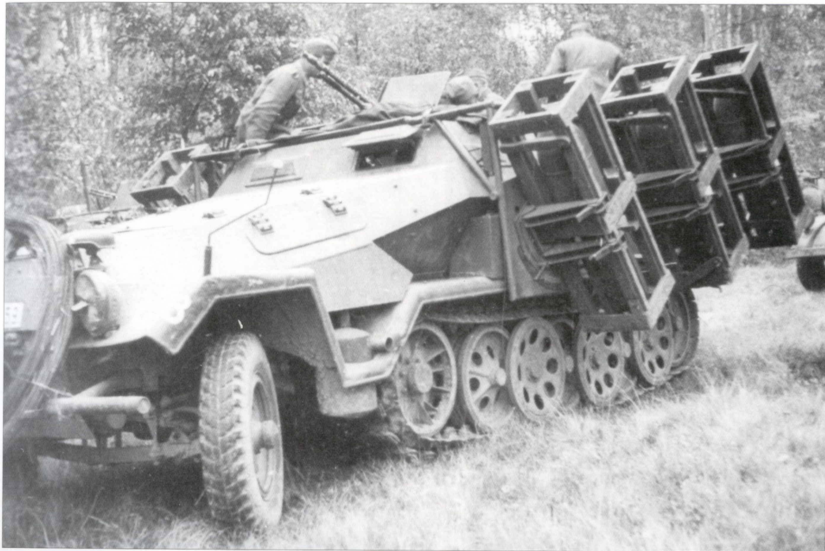
An Sd.Kfz.251/1 Ausf.B with Wurffrahmen. The wooden frames (steel ones were also used) hold the 32 cm Wurfgranate rockets.
