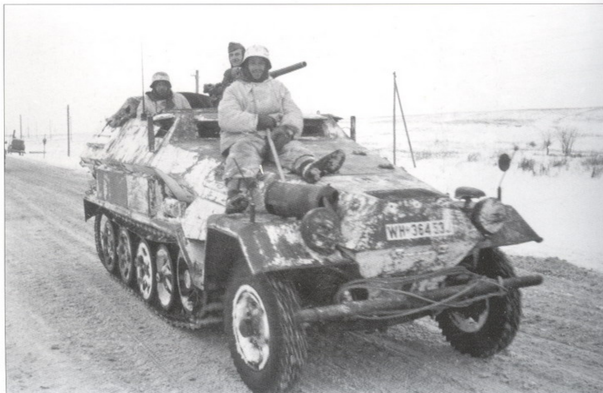
An Sd.Kfz.251/10 Ausf.B on the Eastern Front, winter 1942. Very often the 3.7 cm Pak 36 gun did not have a gun shield.
