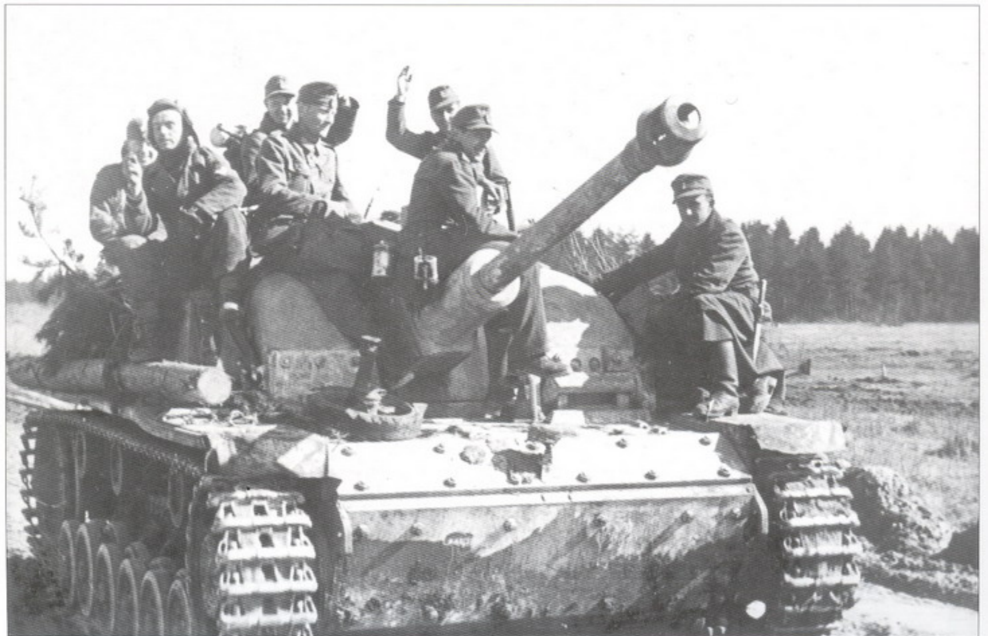
A Sturmgeschütz.III Ausf.G, its front armor reinforced with a layer of concrete. Eastern Front, May 1944.
