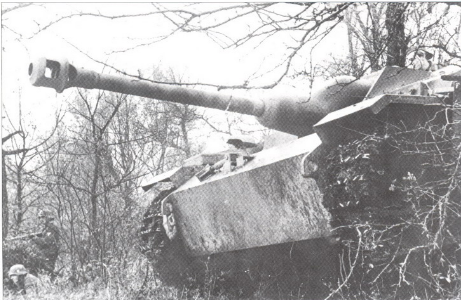
A " Sturmgeschütz.III Ausf.G " belonging to the last production series, in the fall of 1944. Commencing at the beginning of July 1944, a bracket for supporting the gun barrel was sporadically mounted.
