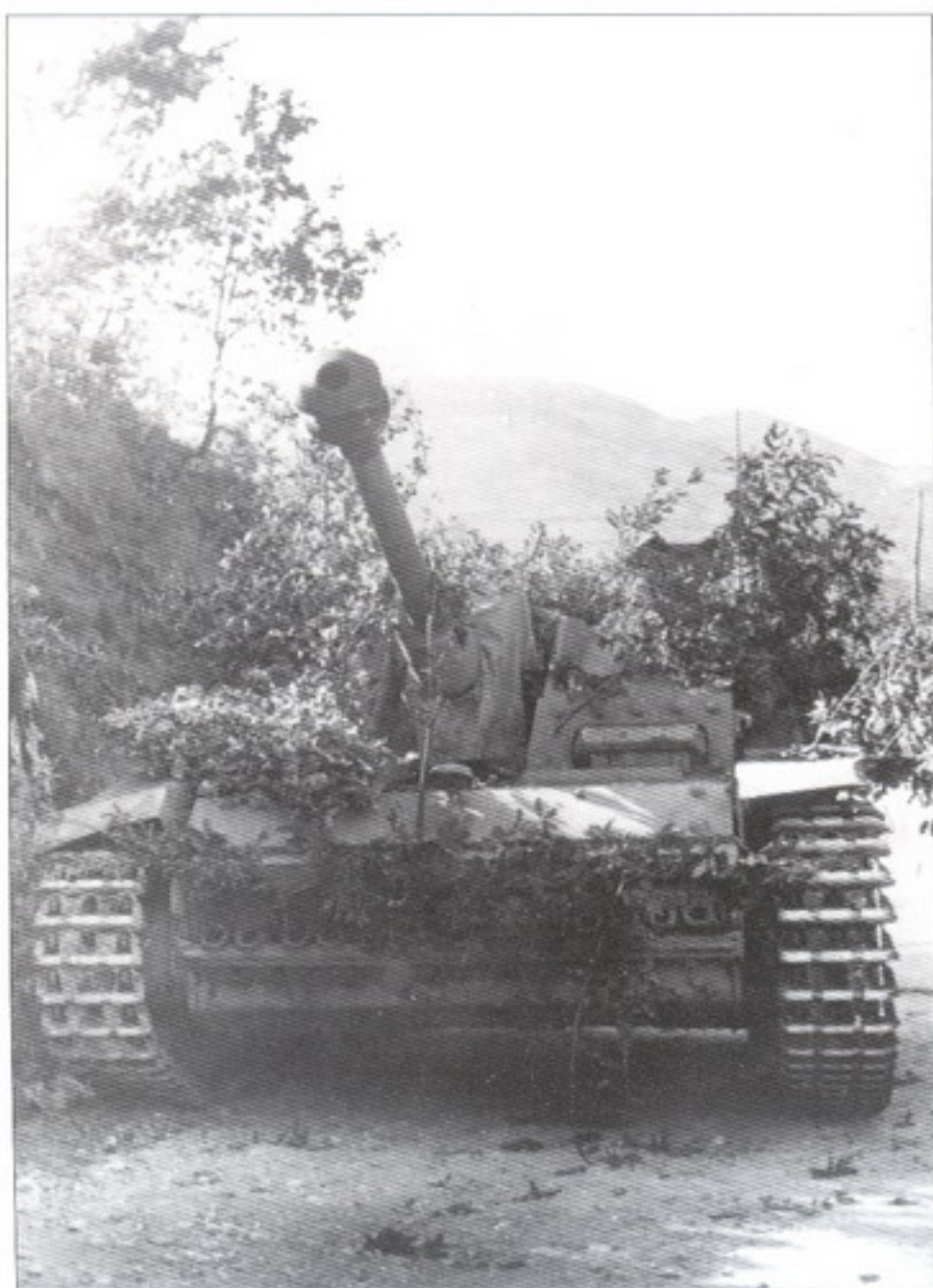
A " Sturmgeschütz.III Ausf.G " belonging to the last production series, in the fall of 1944. Commencing at the beginning of July 1944, a bracket for supporting the gun barrel was sporadically mounted.
