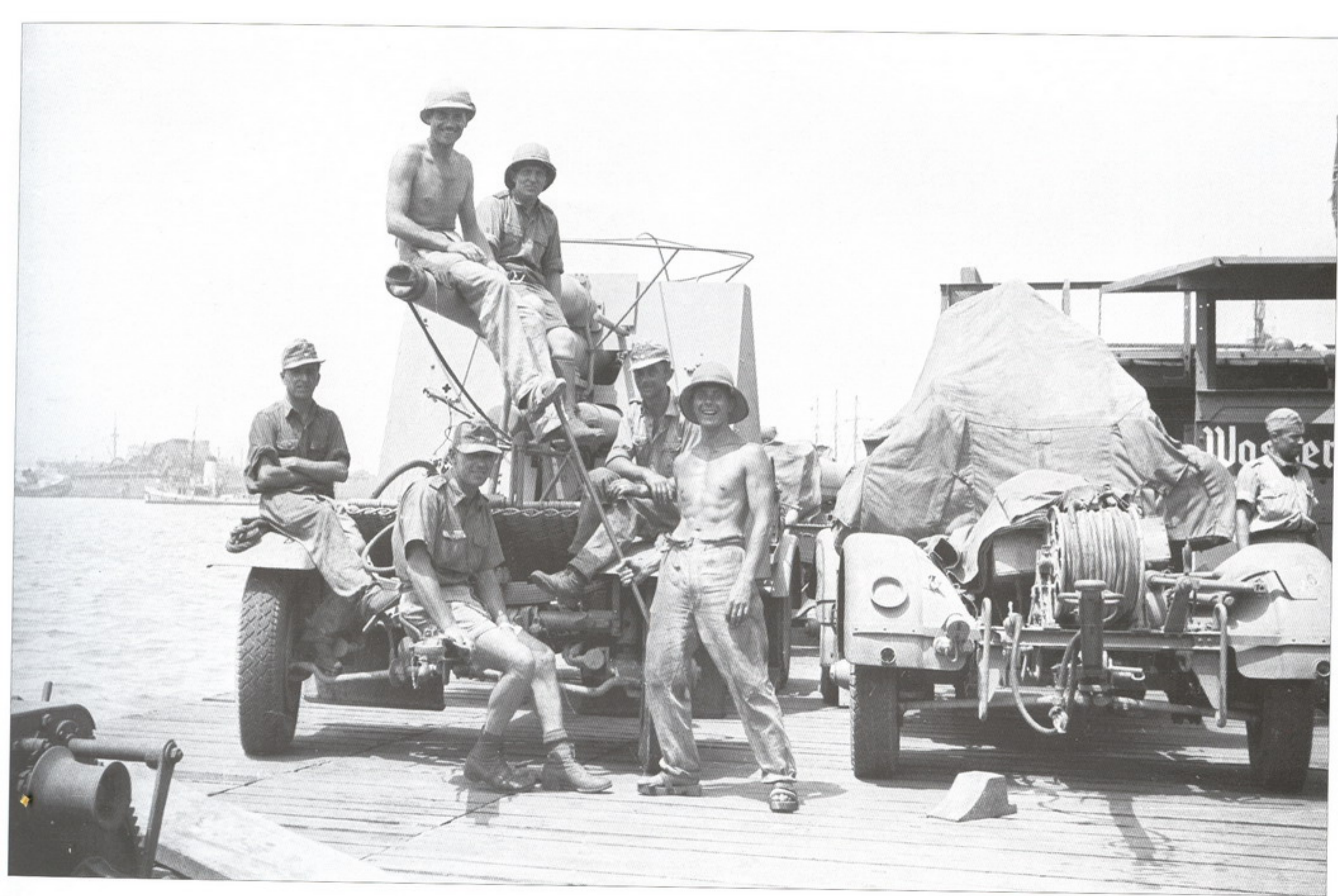
An 8.8 cm Flak 18 reinforcing the Deutsches Afrika Korps. This gun was considered by the Allies as the most dangerous weapon used against their armor. Note the arrangement above the protective shield which allowed for the attaching of camouflage netting.
