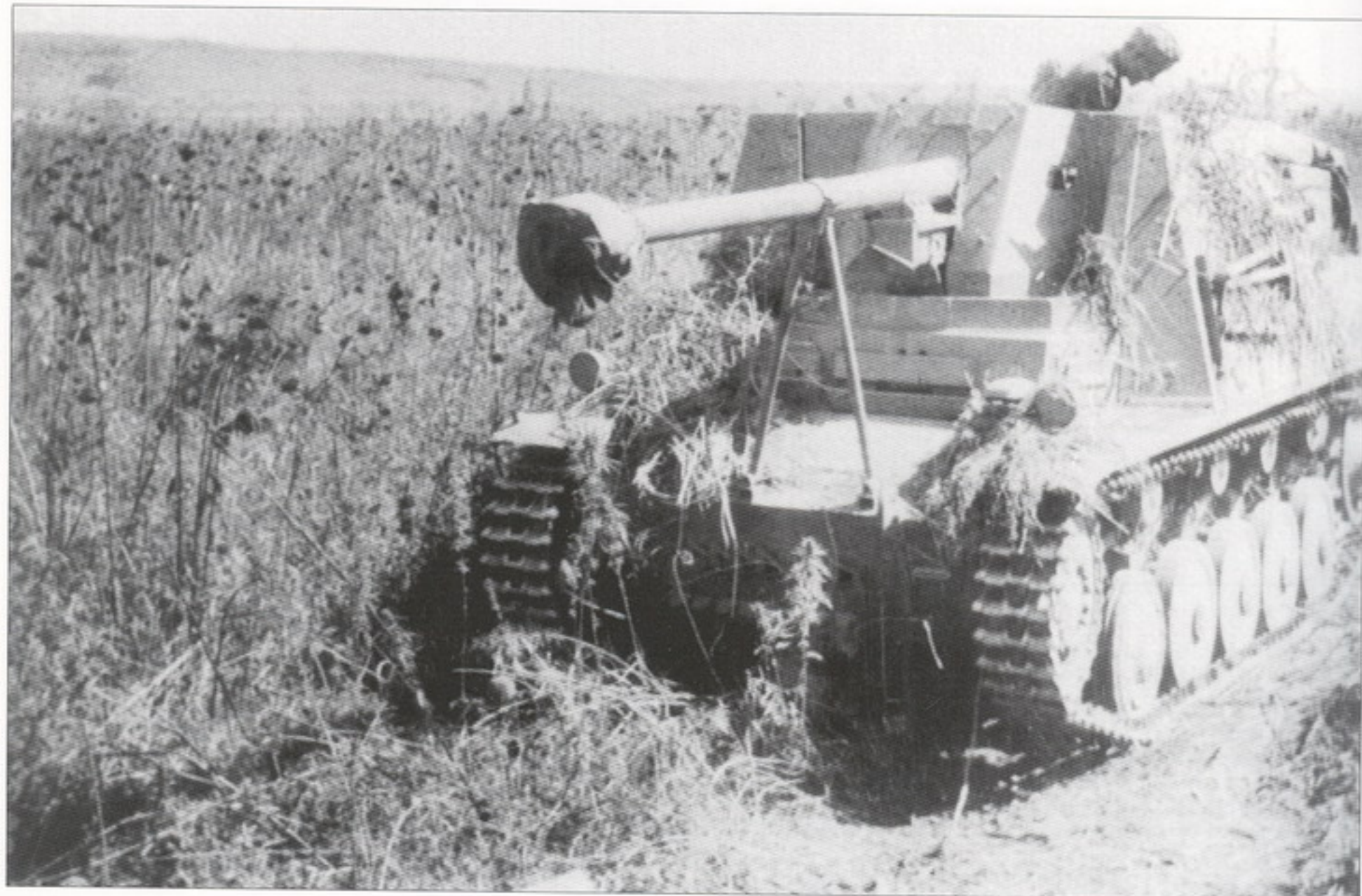
A Marder II (Sd.Kfz.132) 7.5 cm Pak 40 on a Pz.Kpfw.II chassis, on the Eastern Front, 1943.
