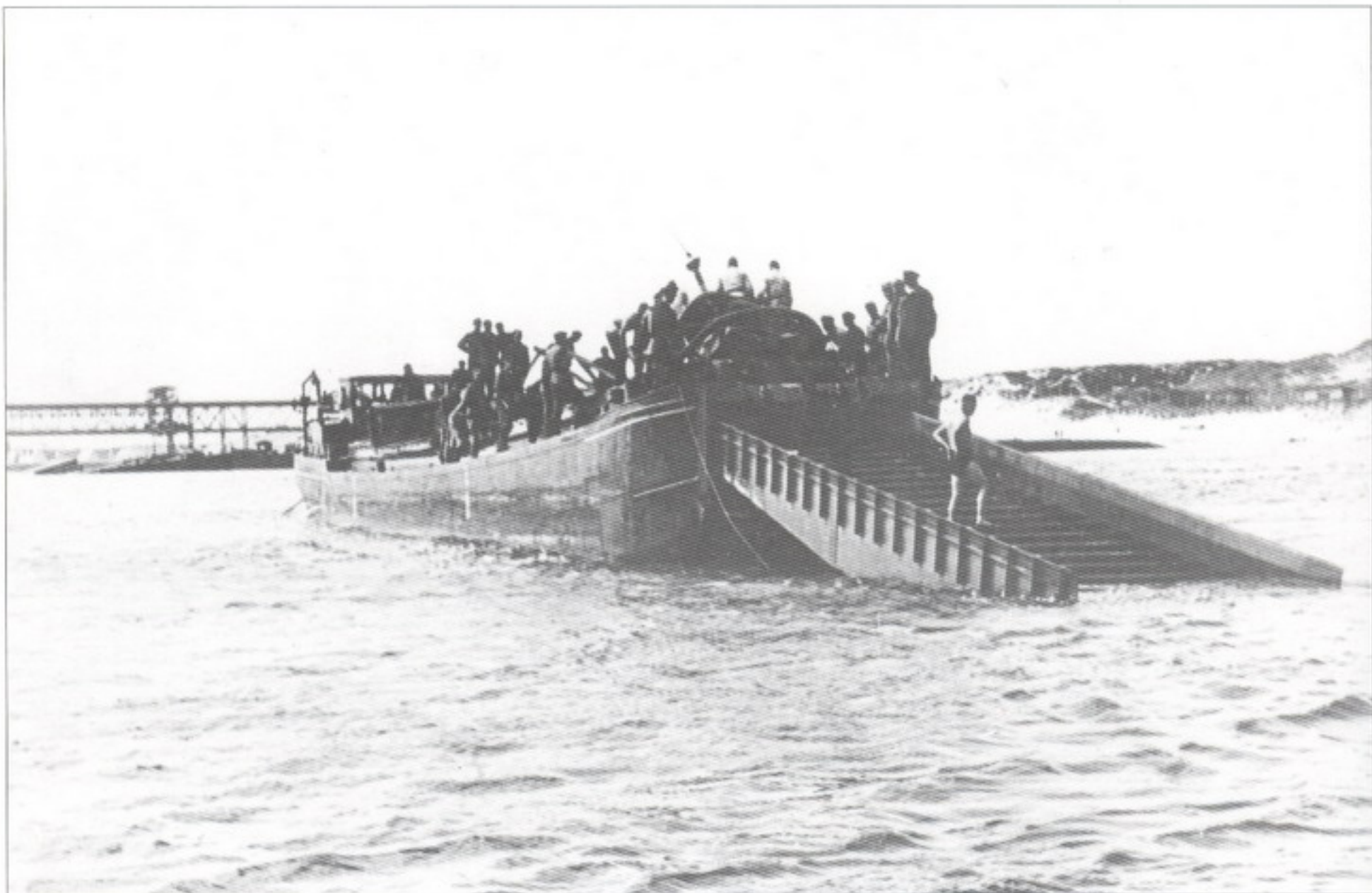
Pz.Kpfw.III Ausf.F (Tauchpanzer) on a Peniche barge equipped with a special Hans Herbert debarking ramp, during training for Operation Sea Lion near the island of Sylt in the Autumn of 1940.
