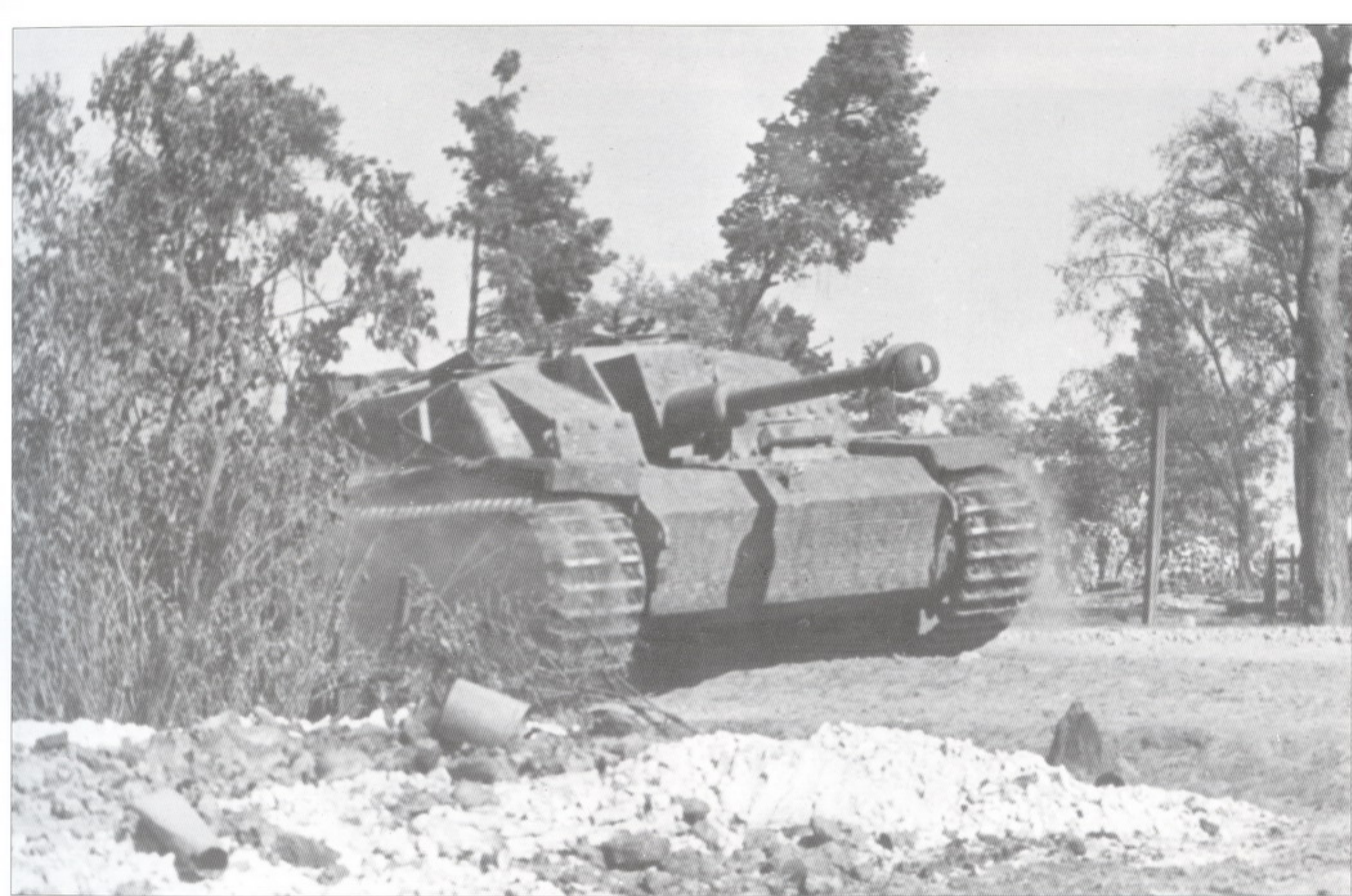
Sturmgeschütz.III Ausf.G of the Sturmgeschütz Kp. of the 18. SS Panzergrenadier Division "Horst Wessel" . A common sight, this vehicle has probably lost its side skirts in action and only the mounting brackets remain. It also has the new type one-piece Ostketten, Eastern Front, summer 1944.
