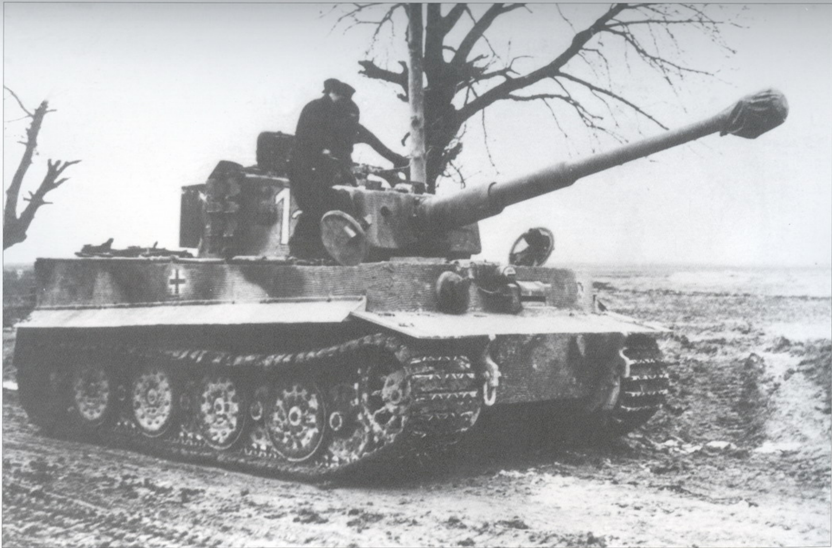
A late production Tiger I (note the steel road wheels) of 1./s.Pz.Abt.507 on the Eastern Front, April/May 1944.
