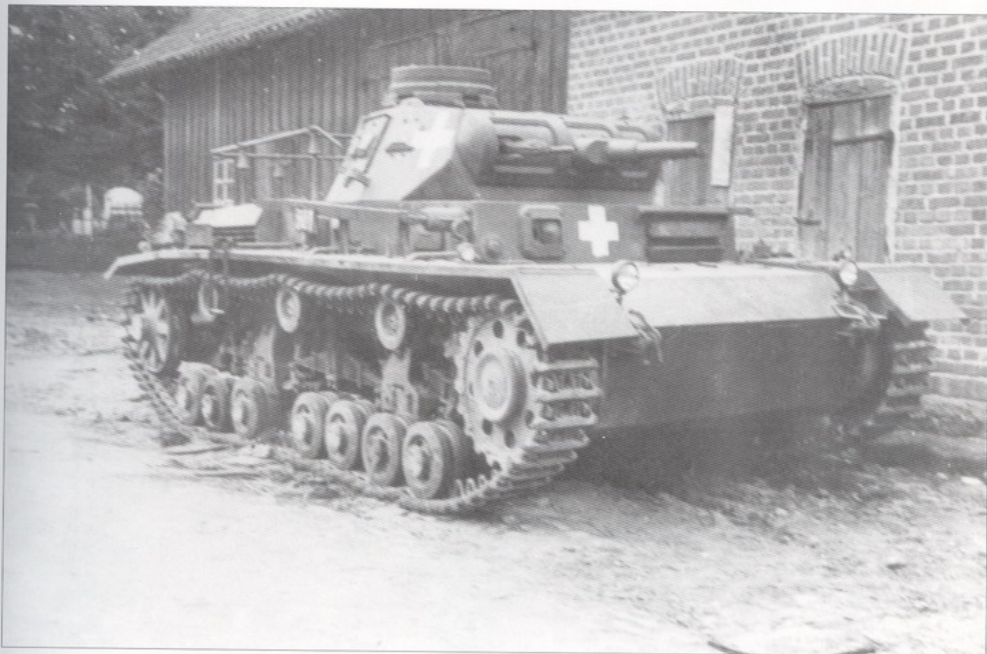
A damaged Pz.Kpfw.III Ausf.D (missing road wheel) during the battles in Poland, September 1939.
