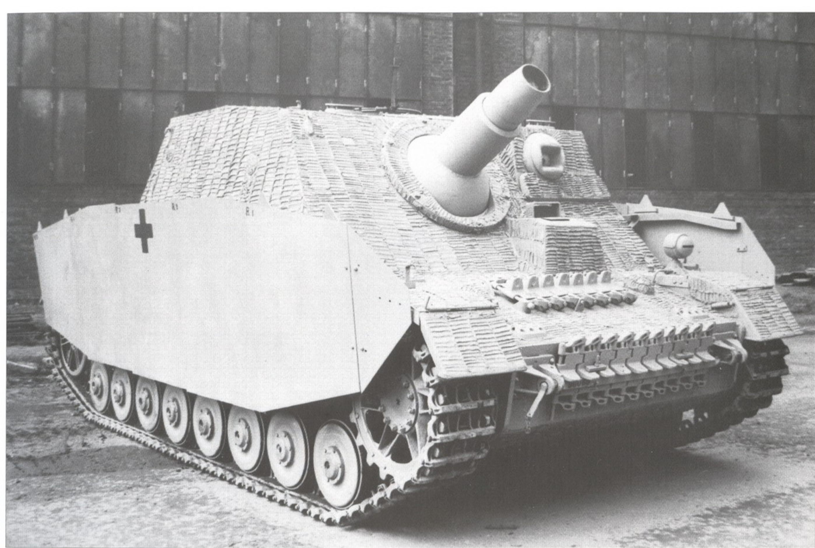
An Sd.Kfz.166 Sturmpanzer 43 from the last production series (the name Brumbär was never used by the Wehrmacht, just by the Allies) with added Zimmeritt.
