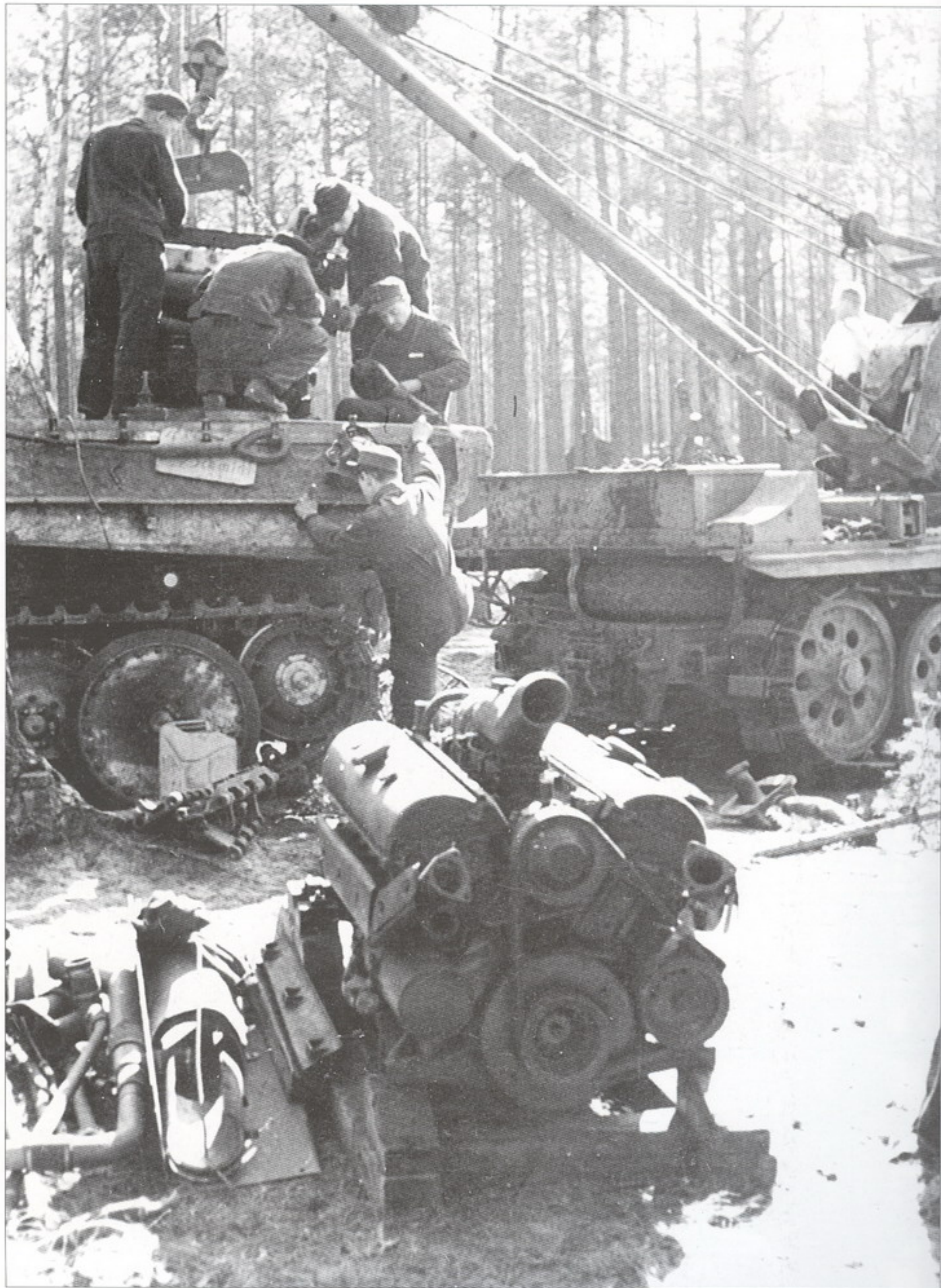
A Panther Ausf.G of Panzer Regiment "Großdeutschland" during repairs, probably in 1945. A 6-ton Bilstein-Drehkran, installed on an Sd.Kfz.9, is being used.
