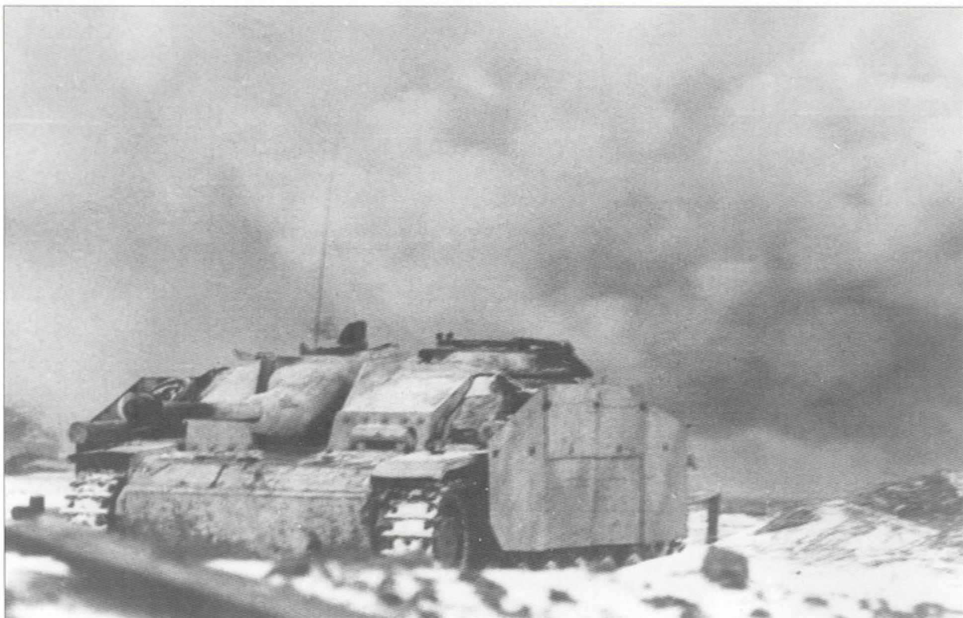
This Sturmgeschütz.III Ausf.G has the Saukopfblende mantlet and the commander's cupola deflector. It is pictured during the battles around Witebsk in February 1944, Army Group Middle.
