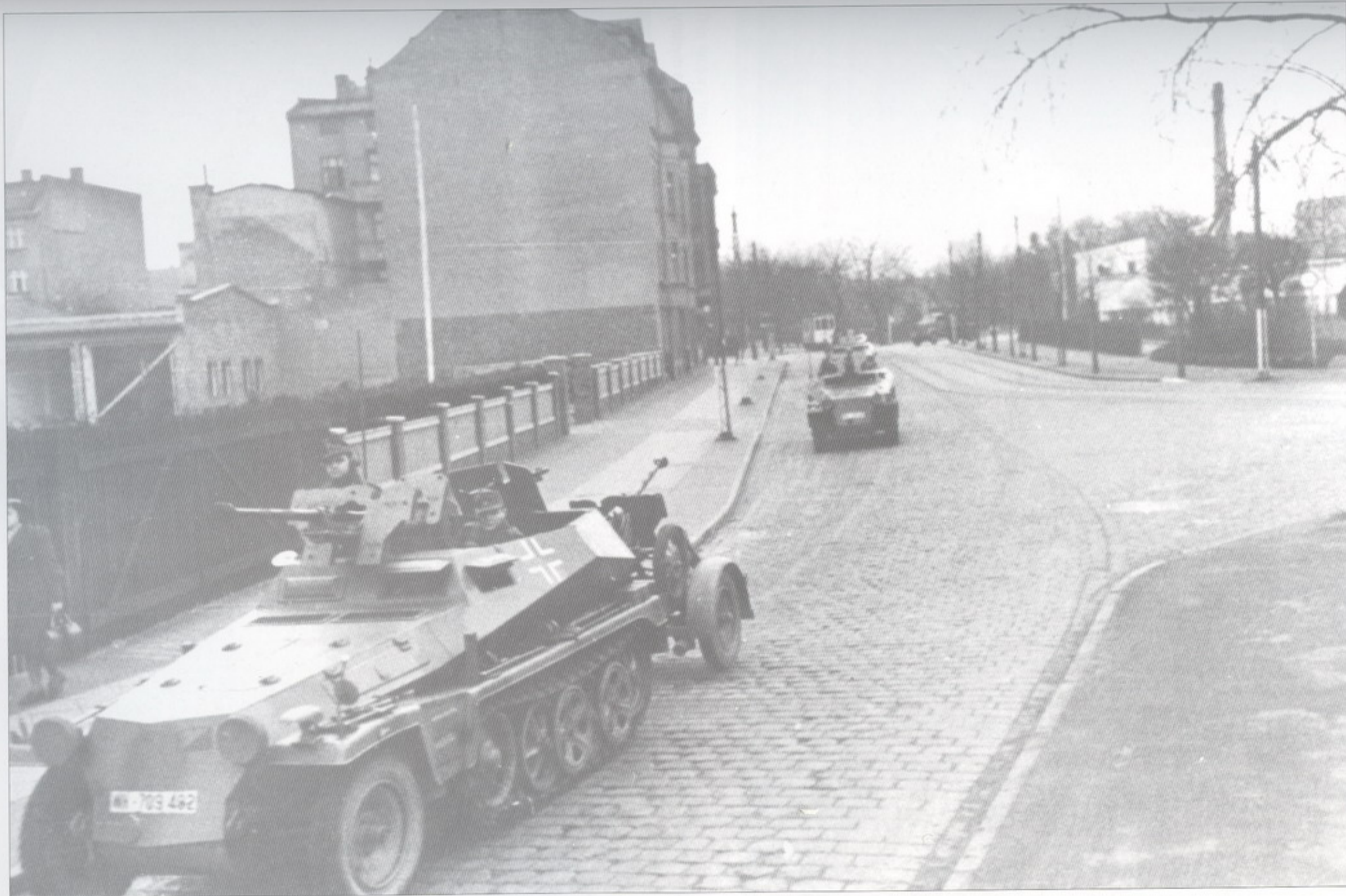
Sd.Kfz.250/11 halftracks (armed with the Pz.B.41 anti-tank rifle) of Aufkl.Abt.580. The method of towing the second anti-tank rifle is certainly unusual.
