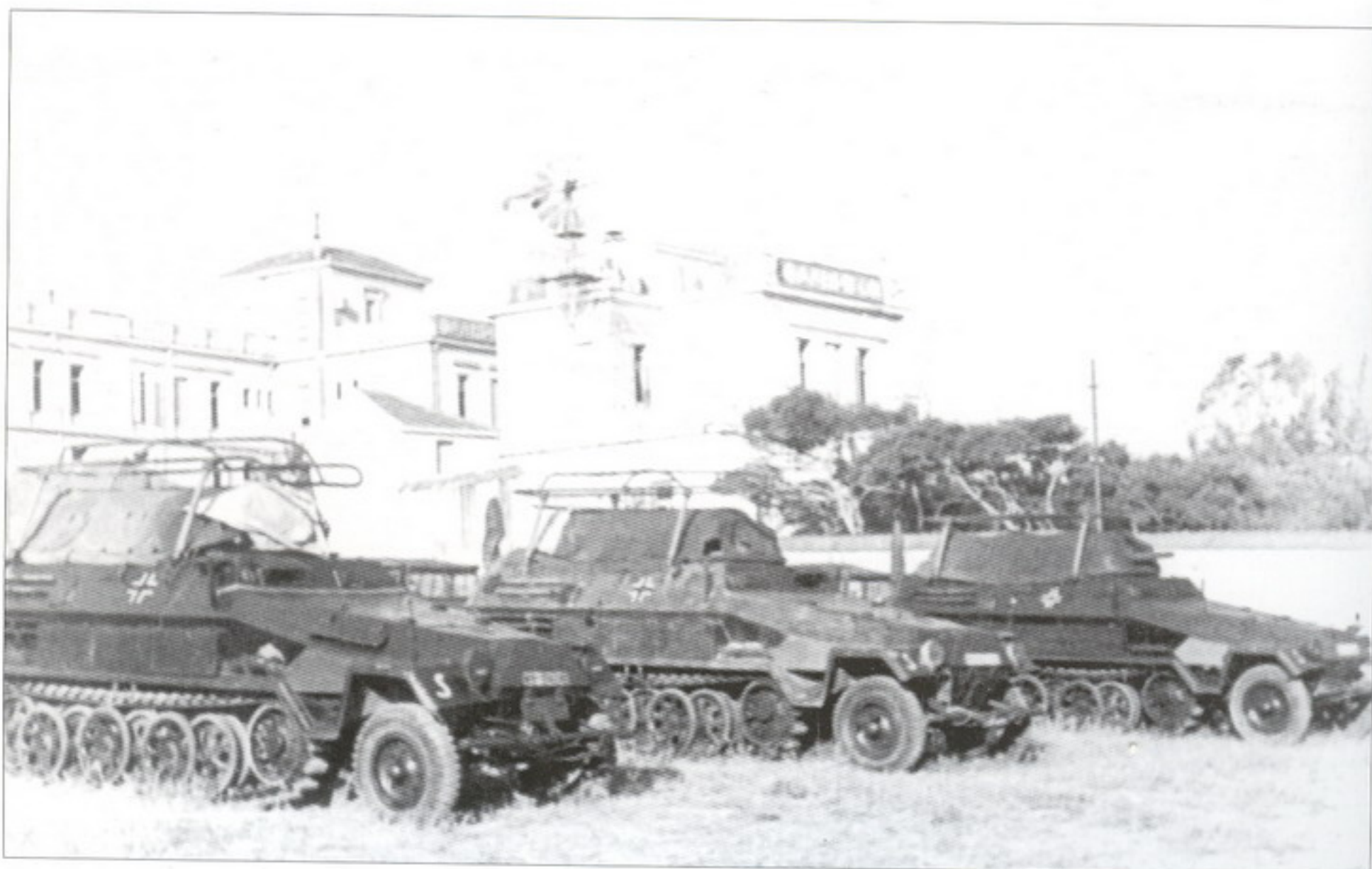
Three Sd.Kfz.251/3 Ausf.B halftracks with the telescopic FuG. 11 masts and tarpaulin covers for the crews, Eastern Front 1941
