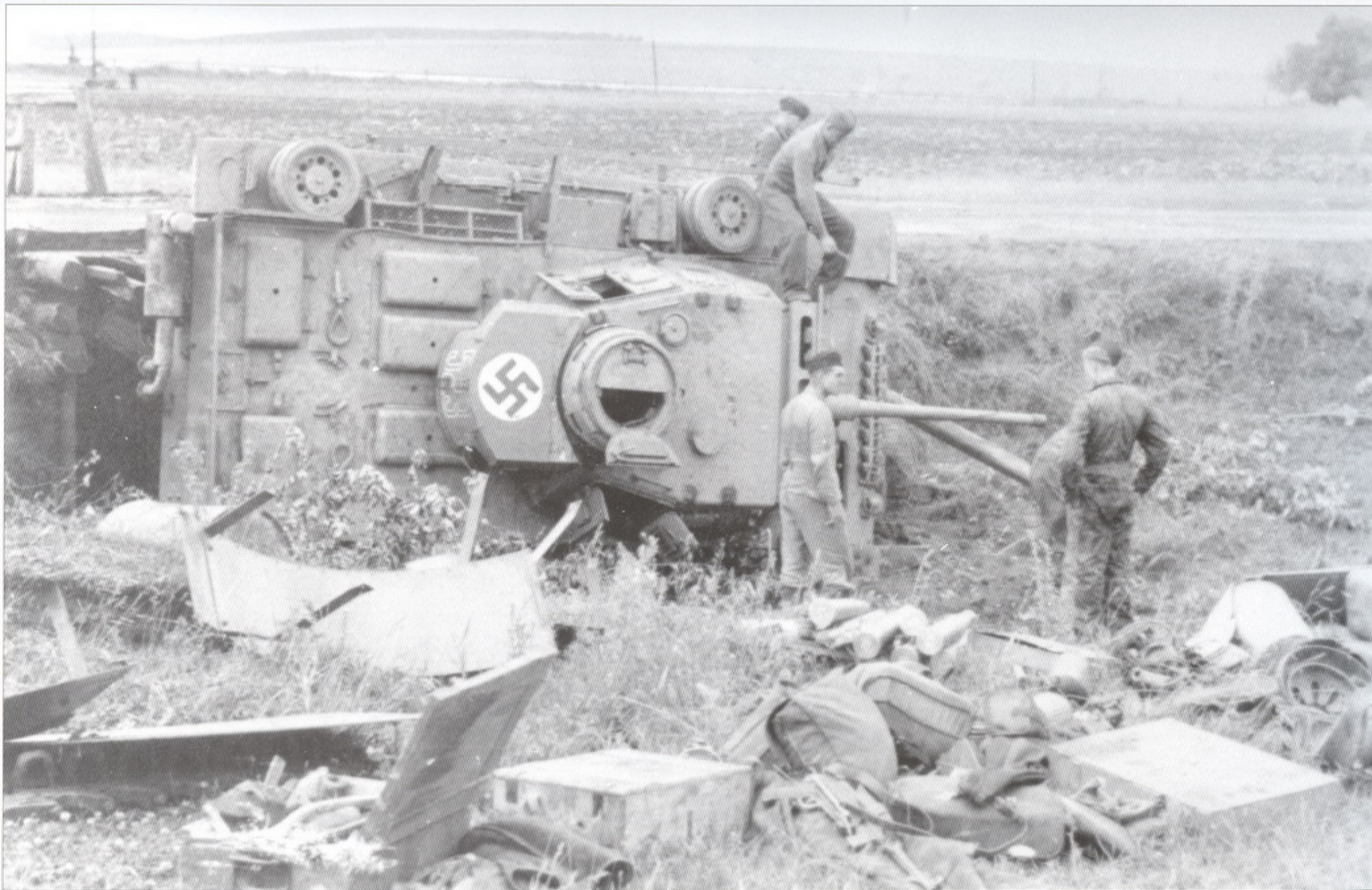
A Pz.Kpfw.III Ausf.M (with the characteristic, for that version, exhaust configuration), probably of SS Panzergrenadier Division "Wiking" , after an accident on a bridge. The unlucky crew has piled up its personal belongings, along with the torn-off turret Schürzen, in the foreground.
