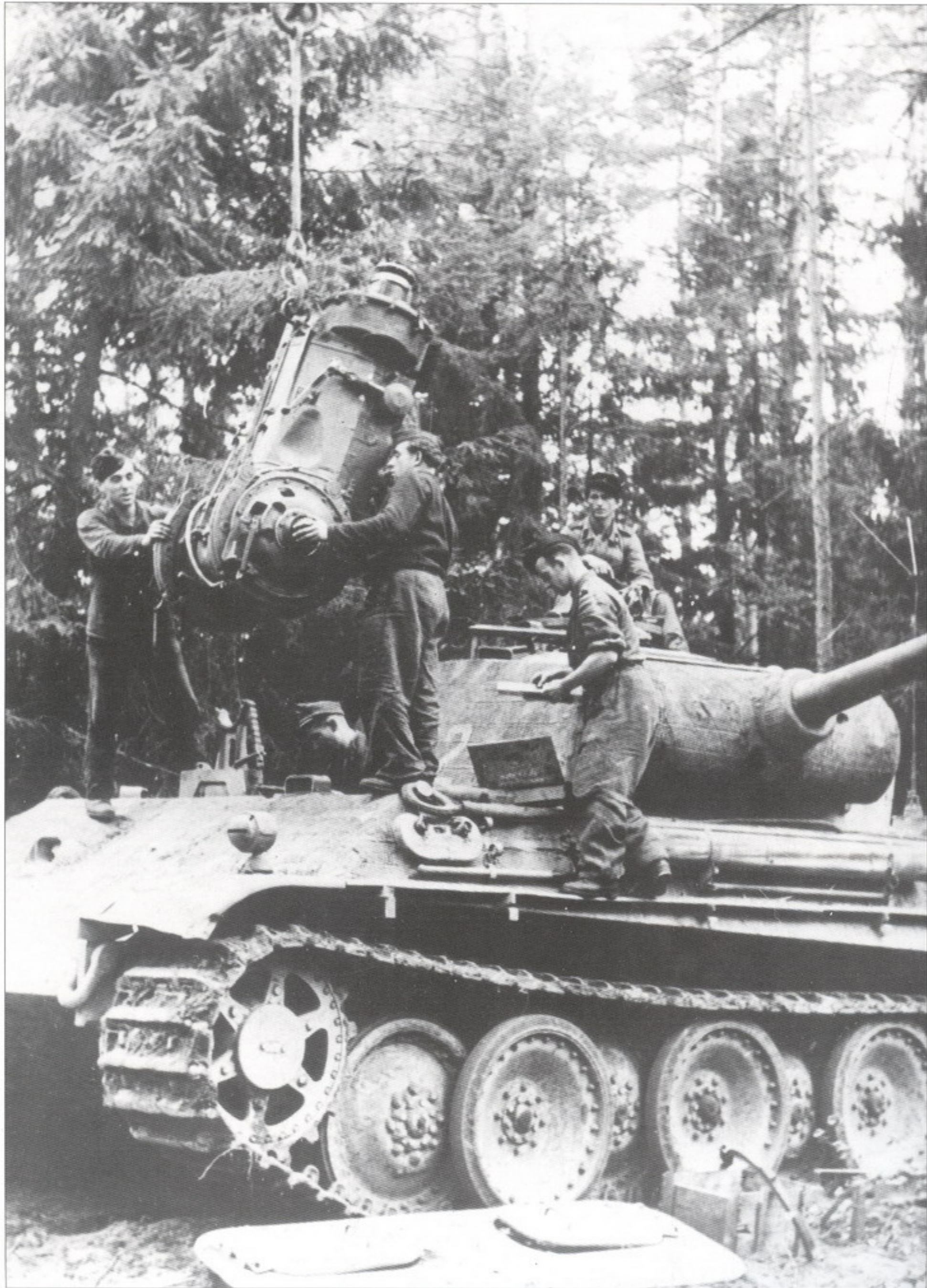
Changing of the transmission on a Panther Ausf.G (Befehlswagen Sd.Kfz.267) in 1944.
