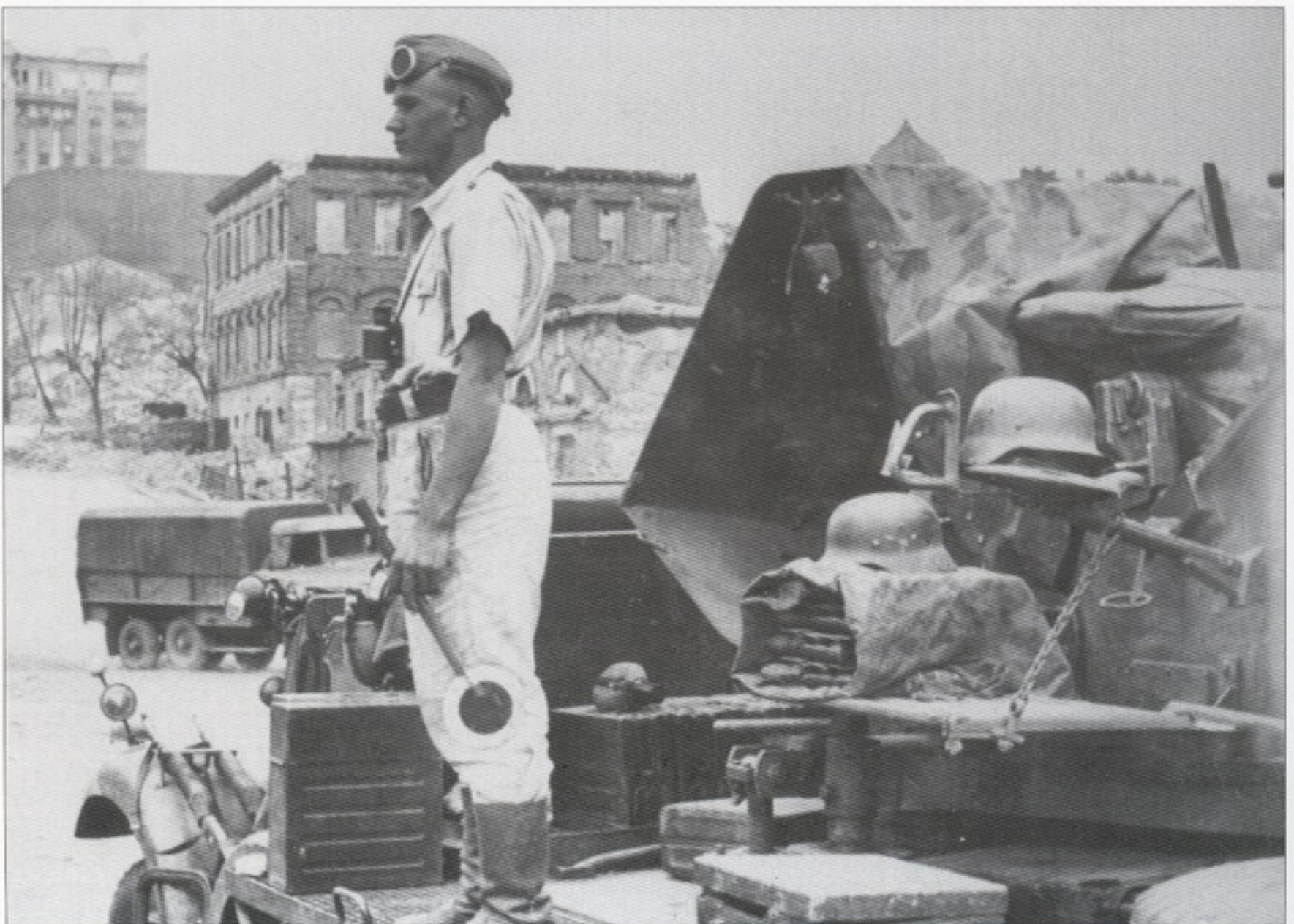
An Sd.Kfz.7 with a partially armored superstructure serving as a prime mover for a special version (socalled Bunkerflak) of an 8.8 cm Flak . The Flak has an enlarged gun shield installed.
