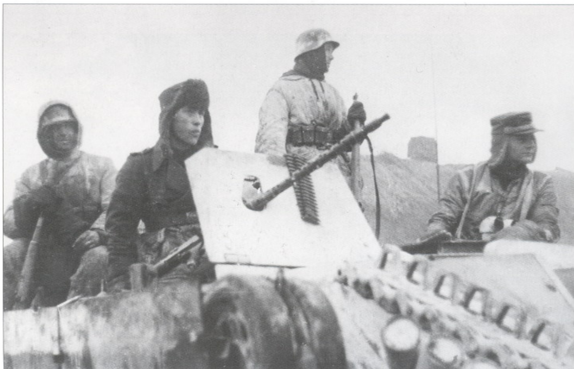
This Sturmgeschütz.III Ausf G was produced between Feb. and May 1943, as evidenced by the presence of the mounted smoke candle launchers (Nebelkerzen-Wurfgerät). Eastern Front, winter 1943-44.
