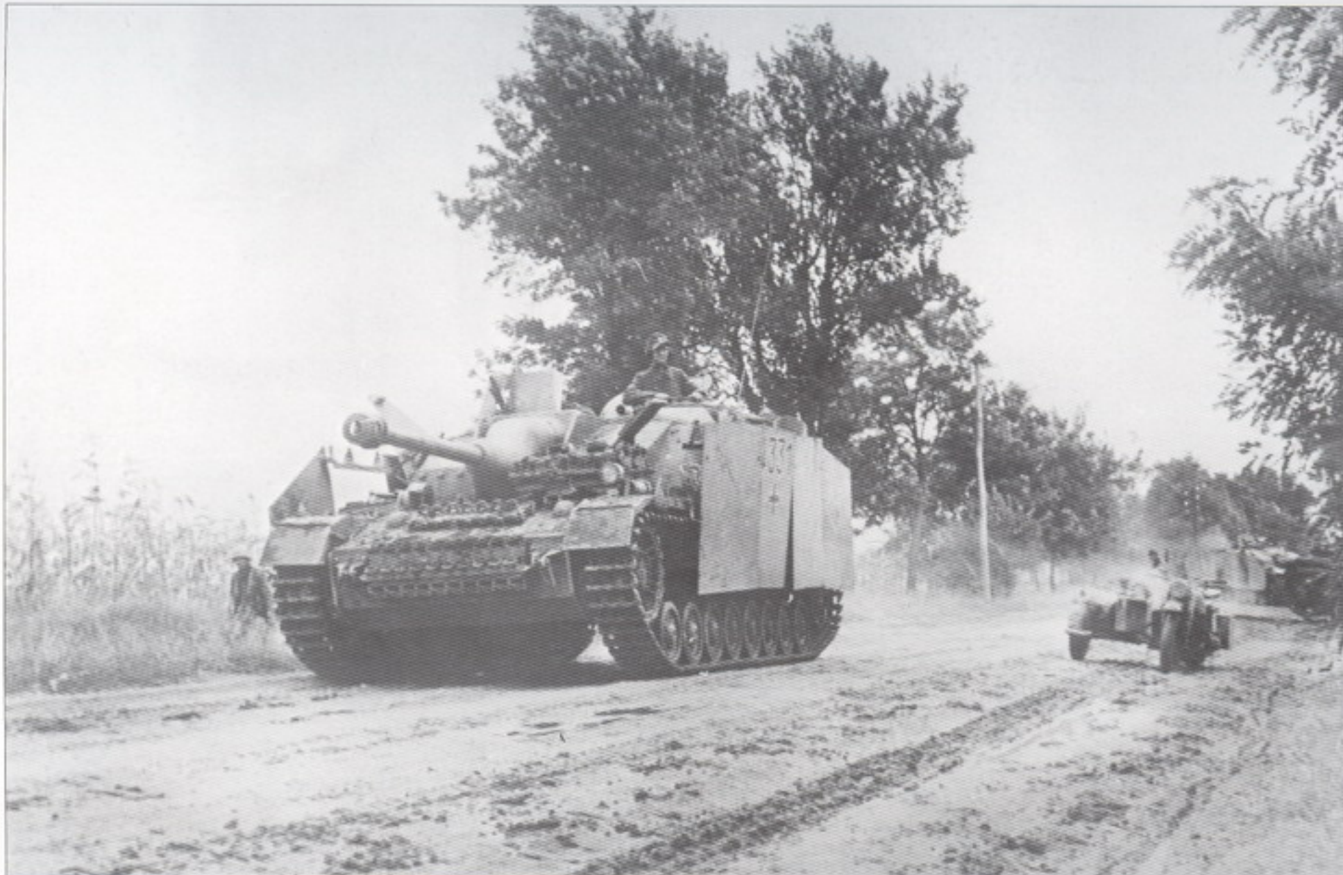
This Sturmgeschütz IV belongs to SS-Sturmgeschütz Abt. 4 of the 4. SS Panzergrenadier Division, "Polizei" , Hungary, November 1944. It has spare track links as added armor protection for the driver.
