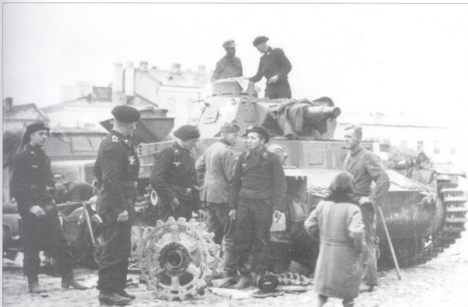
Repairing the differential and a drive sprocket on a Pz.Kpfw.IV Ausf.A in Poland, September, 1939.
