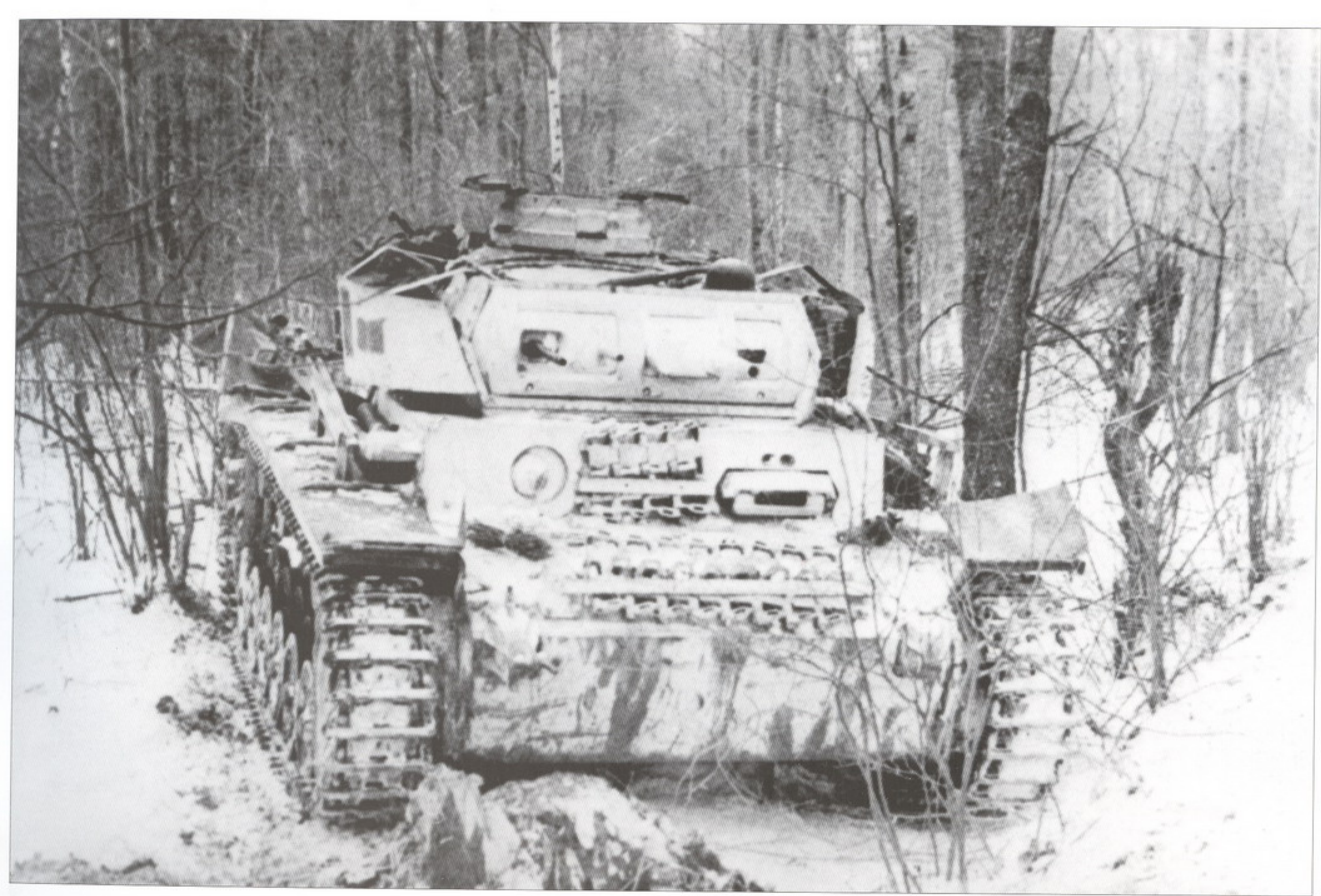
A Pz.Kpfw.III Ausf.H (Befehlswagen) of 5.Panzer Division, Eastern Front, winter 1942. It is armed with only one MG 34, the second one is a dummy.
