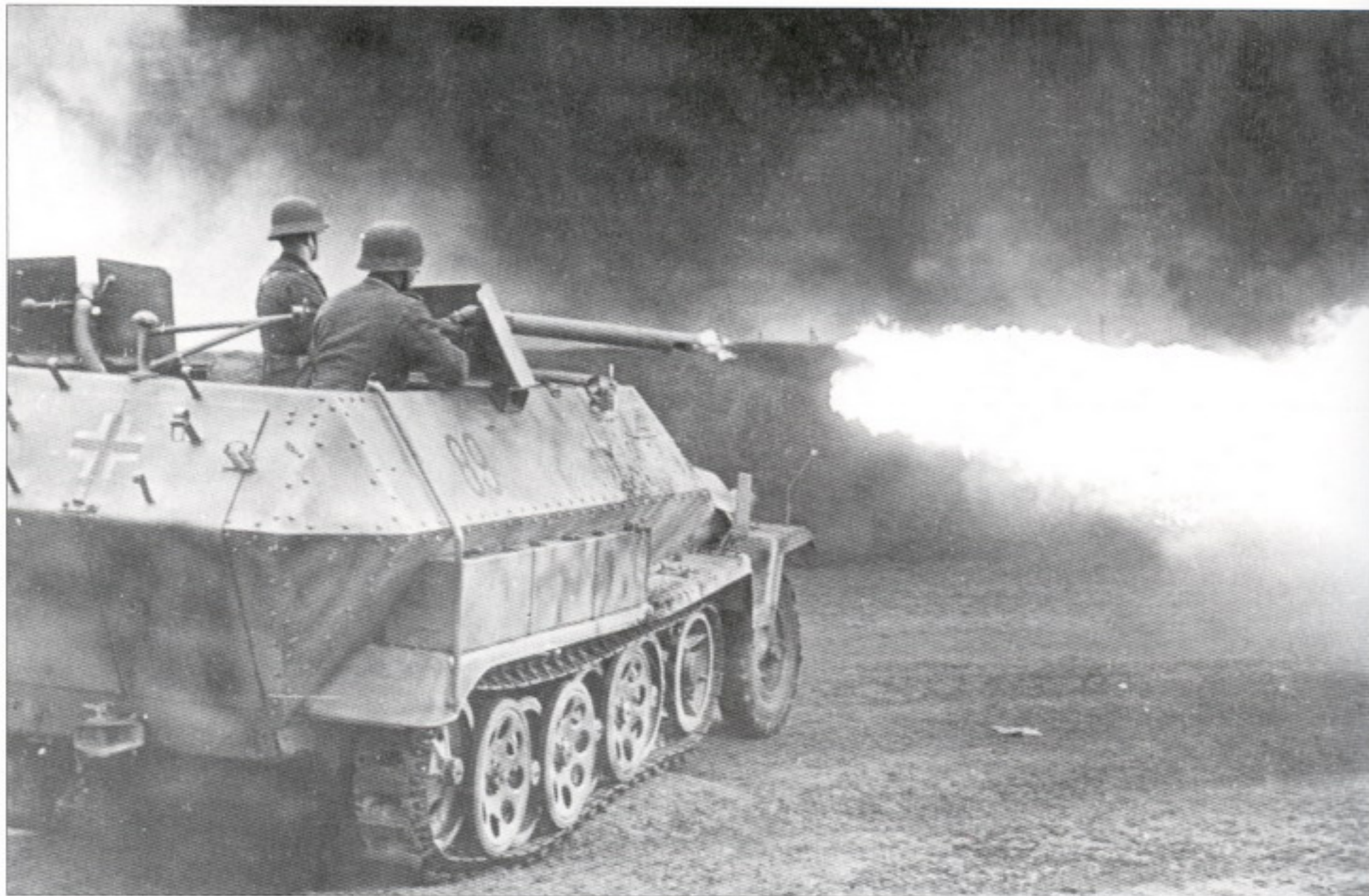
This Sd.Kfz.251/16 Ausf.C ( mittlerer Flammpanzerwagen ) is firing with only one of its two flamethrowers. It had a range of up to 60 meters and also carried a third, portable flamethrower.
