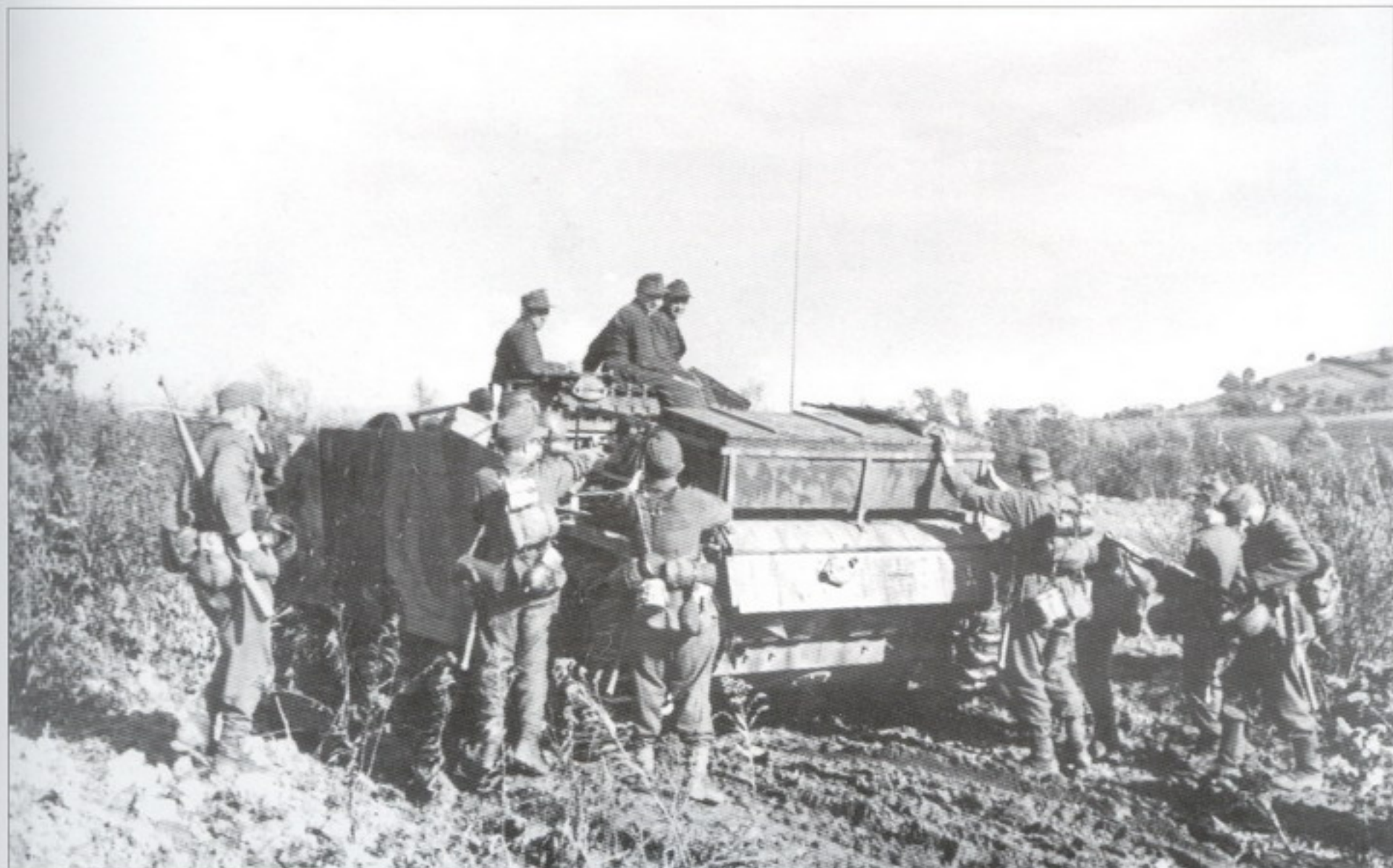
This Sturmgeschütz.III Ausf.G has the characteristic tubular steel rack for stowing additional equipment over the engine deck. Eastern Front, 1944.
