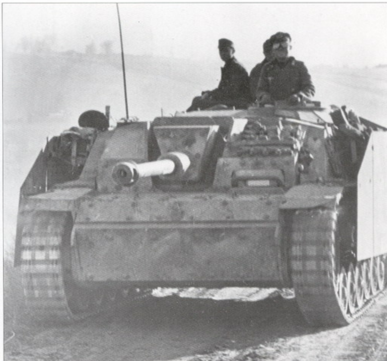
The crew of this Sturmgeschütz. Ausf.G has mounted spare track links as extra protection for the driver. Eastern Front, 1943.
