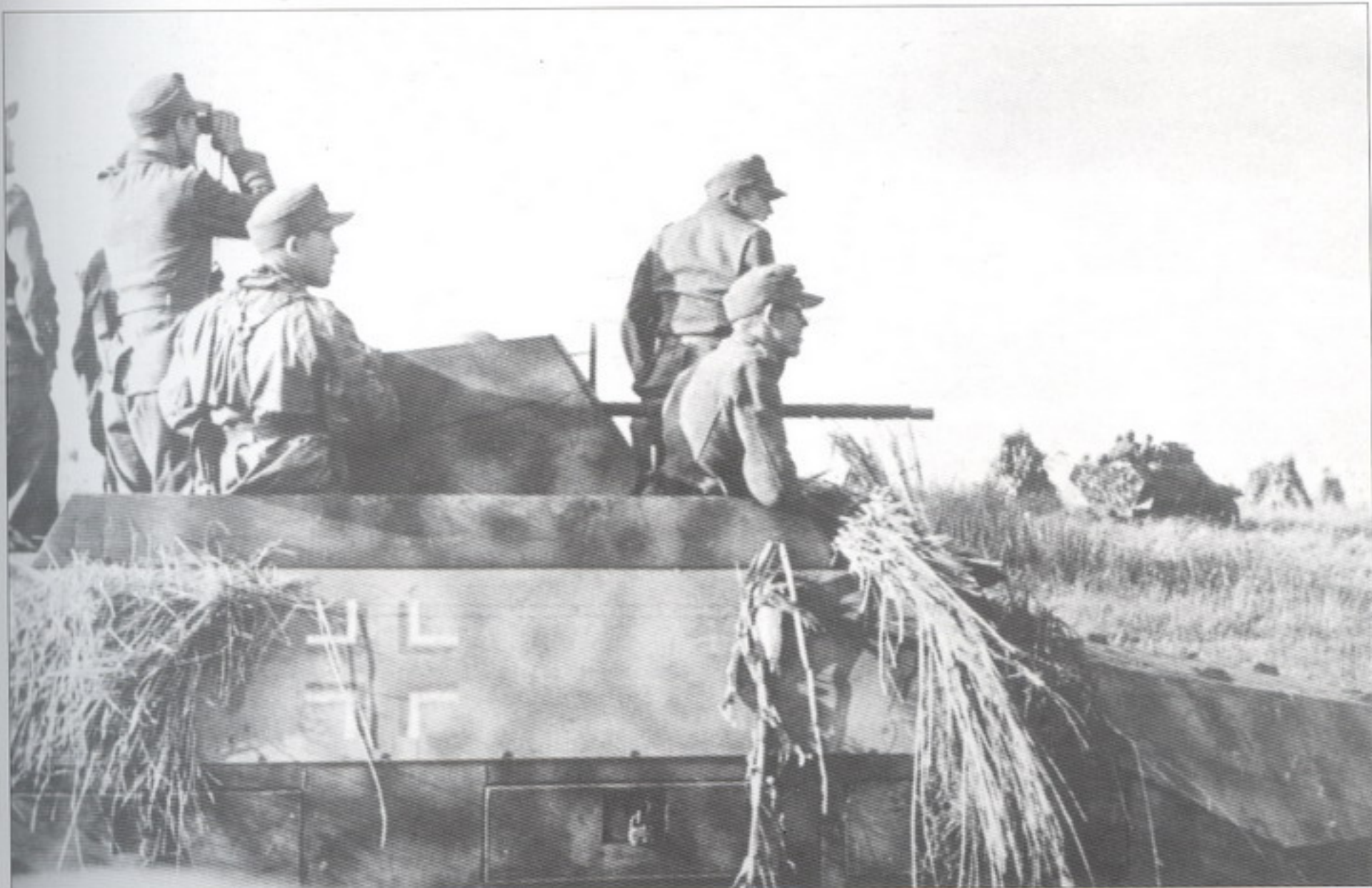
An Sd.Kfz.251/21 Ausf.D ( mittlerer Schützenpanzerwagen mit Drilling MG 151 ) armed with three MG 151 guns (these were mostly of 2 cm caliber, but the 15 mm was also used occasionally). This arrangement was mounted on the gun carriage and had a gun shield as protection for the crew. This vehicle carried 3,000 rounds of ammunition as its standard load.
