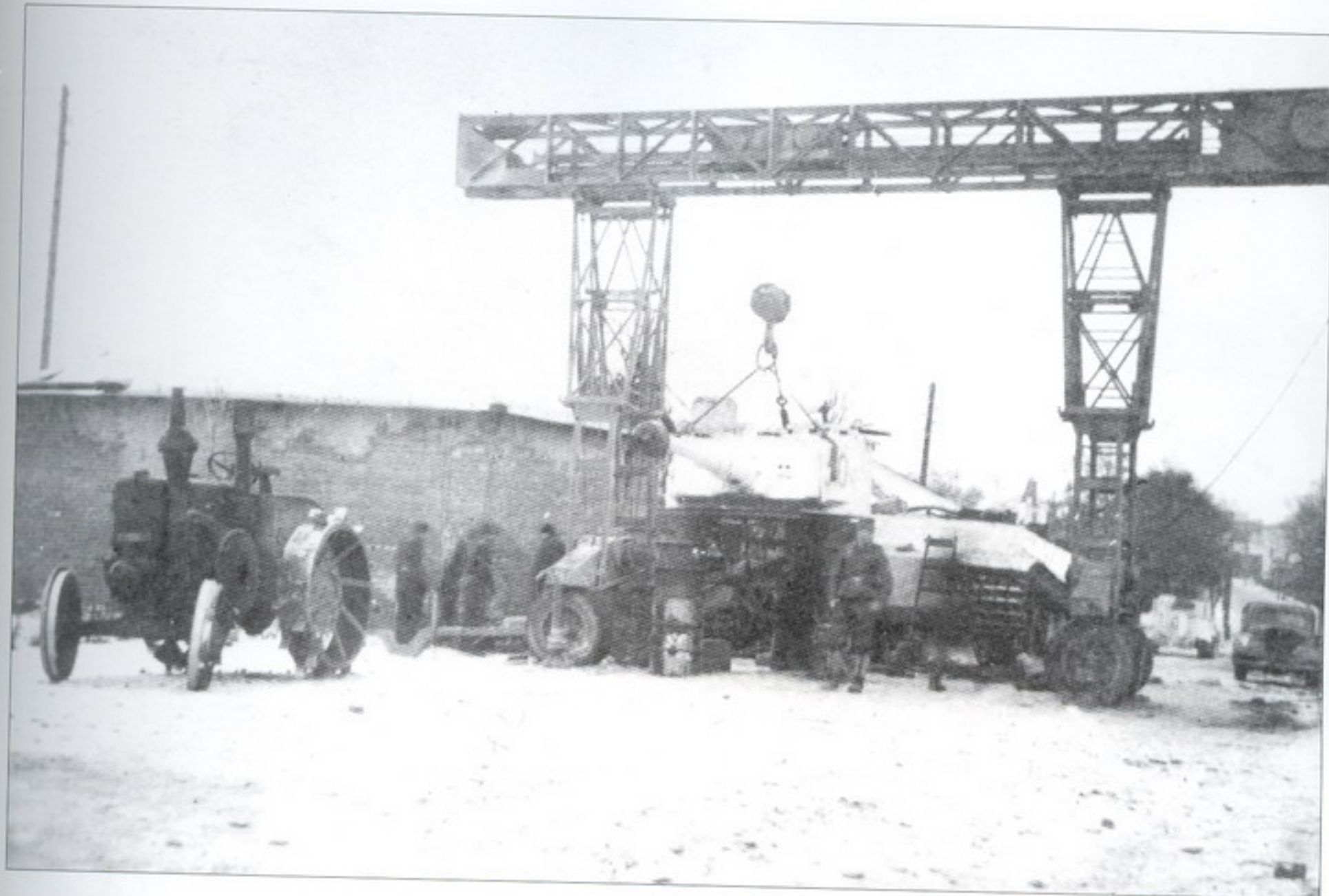
A Tiger on the Eastern Front being repaired and after repairs by the Werkstatt company. Serious repairs of Tigers and Panthers (especially when working on the turret) required the use of the " Fries " 16 ton portable crane.
