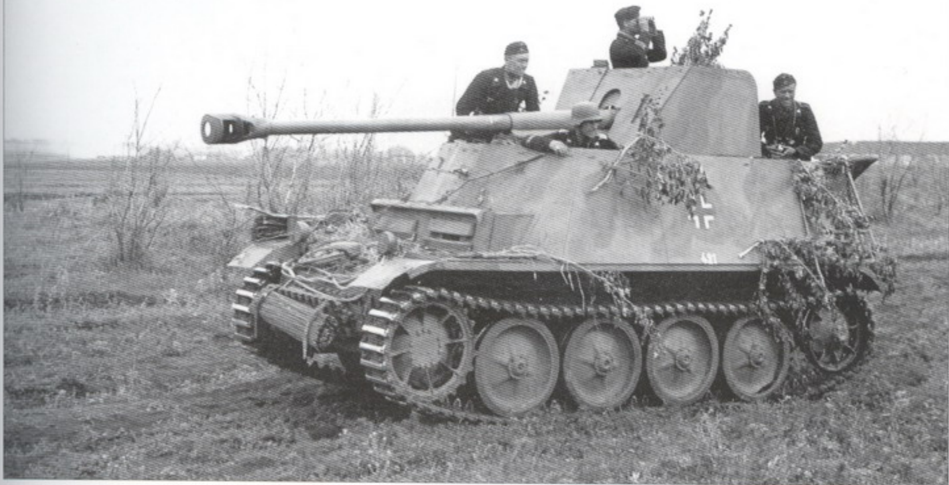
A Marder II (Sd.Kfz.132 armed with a 7.62 cm Pak (r) on a Pz.Kpfw.II Ausf.D chassis) on the Eastern Front , 1942.
