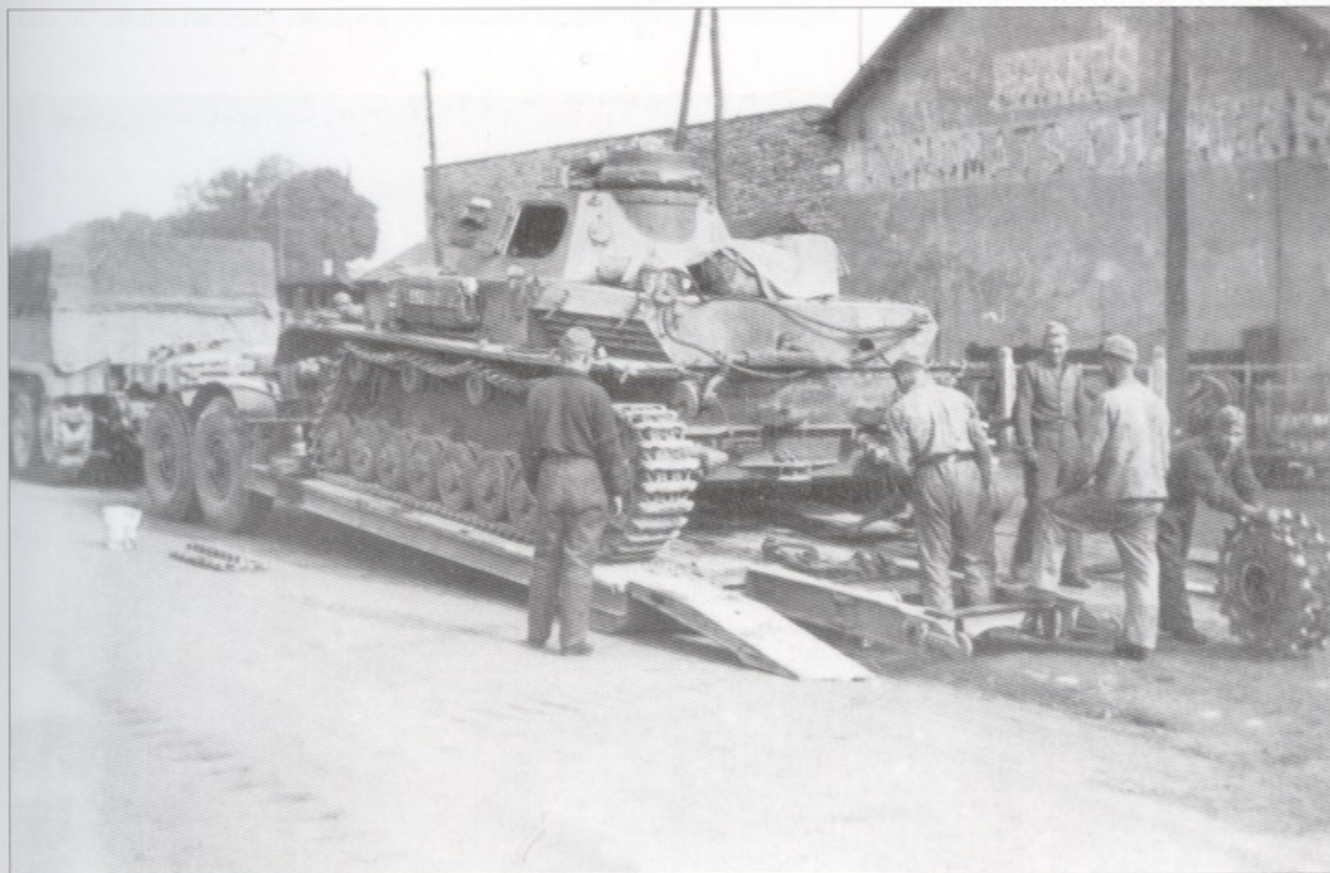
A damaged Pz.Kpfw.IV Ausf.C on a Tiefladeanhänger Sd.Ah.116 trailer, being towed by an Sd.Kfz.9 on the Western Front, 1940.
