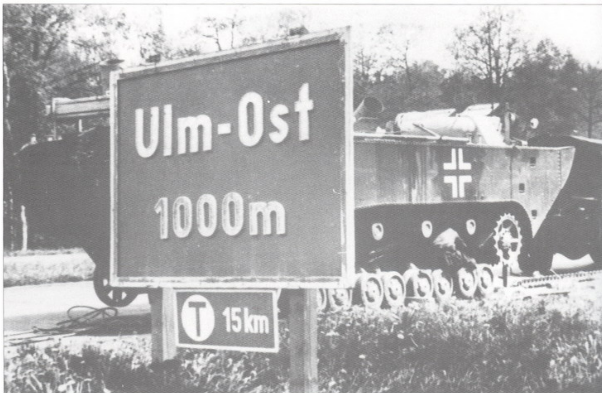
An LWS II during trials, obviously there is a problem with the drive sprocket
