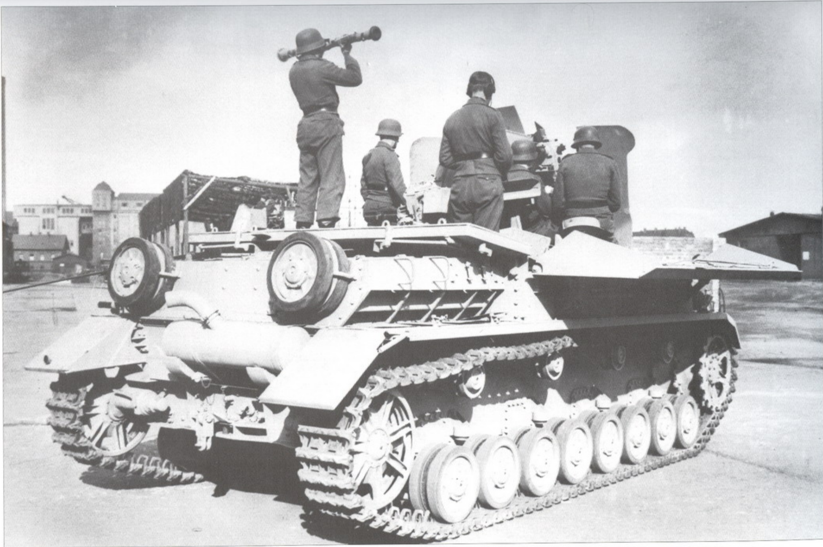
An Sd.Kfz.163/3 Möbelwagen with its side armor panels lowered and its crew ready to fire.
