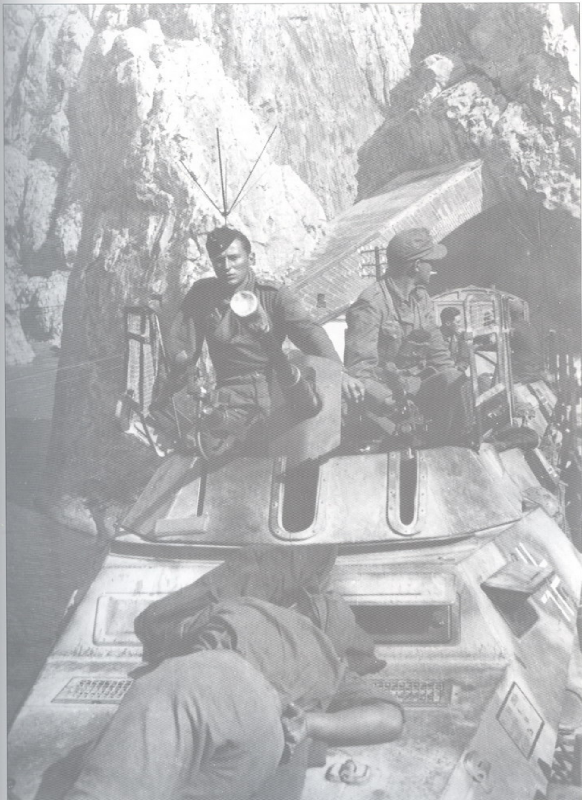
An Sd.Kfz.250/9 (armed with a 2 cm Flak 38 ) in Greece. The installed Sternantenne D suggests that the vehicle houses an extensive set of radio equipment.
