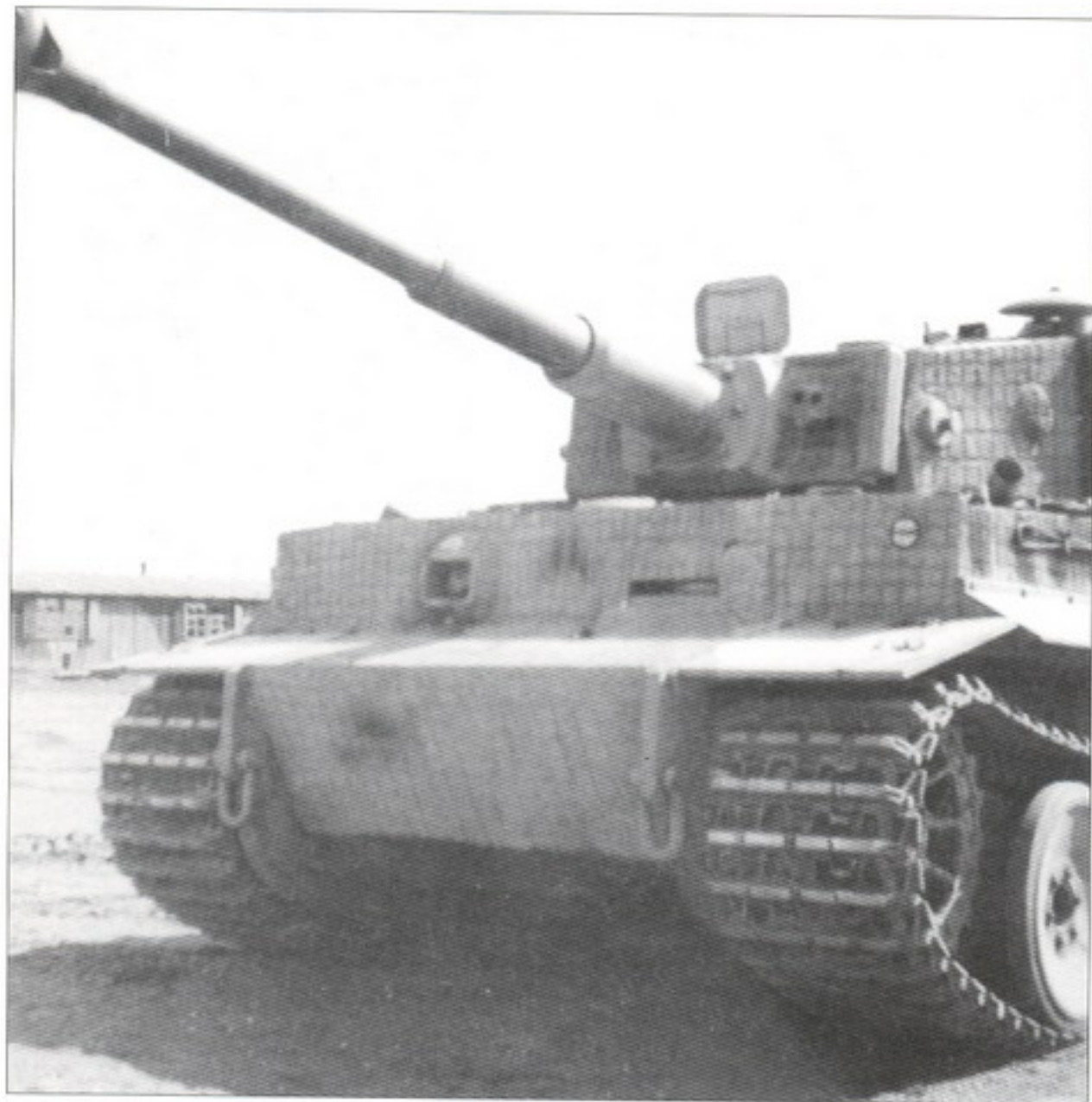
Tiger I , probably of Pz.Ers.Abt.500 , powered by natural gas.
