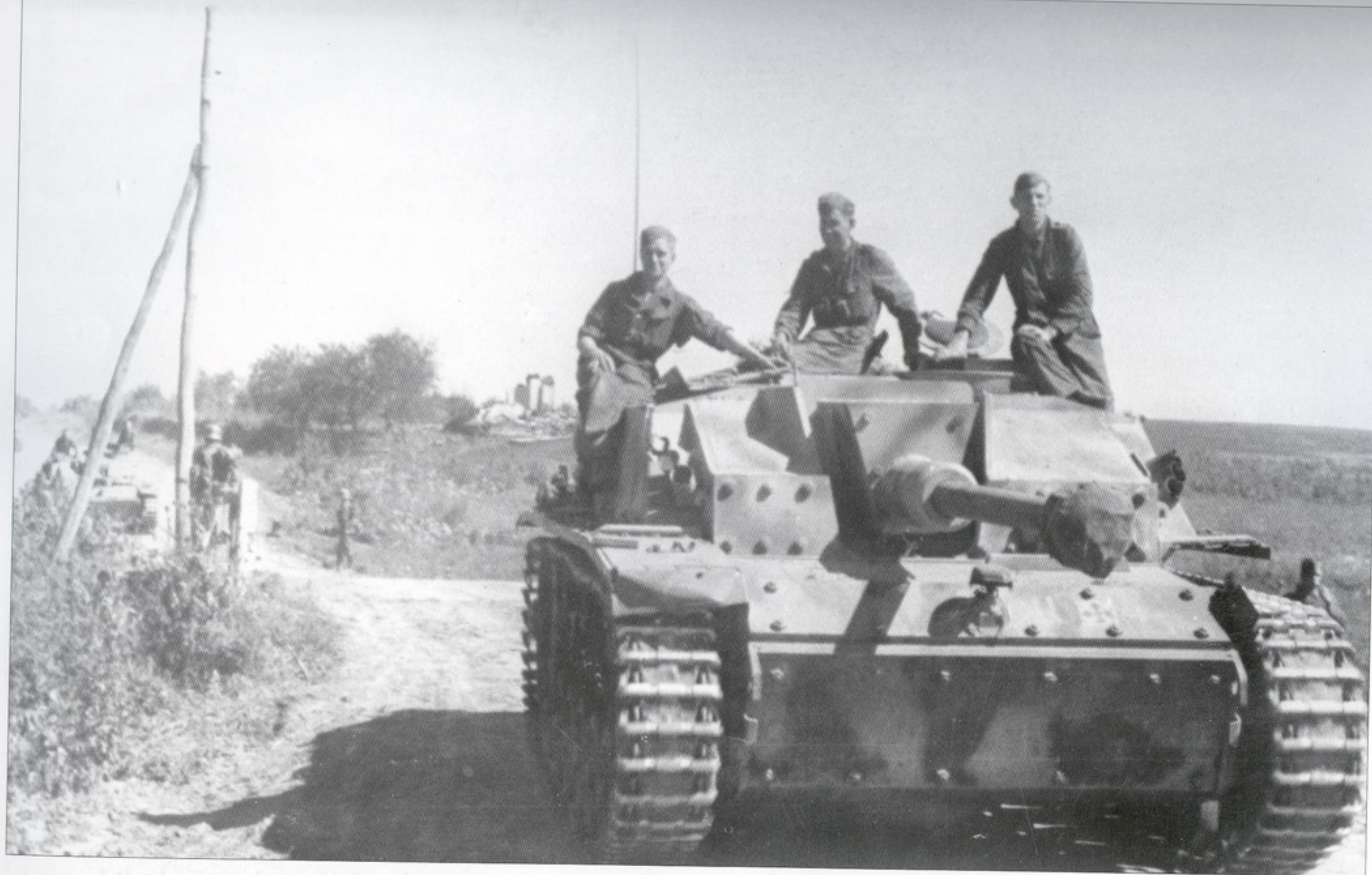
A Sturmgeschütz.III Ausf.G produced between February and March 1943, as evidenced by the presence of mounted smoke candle launchers. This vehicle belongs to the Sturmgeschütz Batterie of 2 SS Panzerdivision "Das Reich", Eastern Front, August, 1943.
