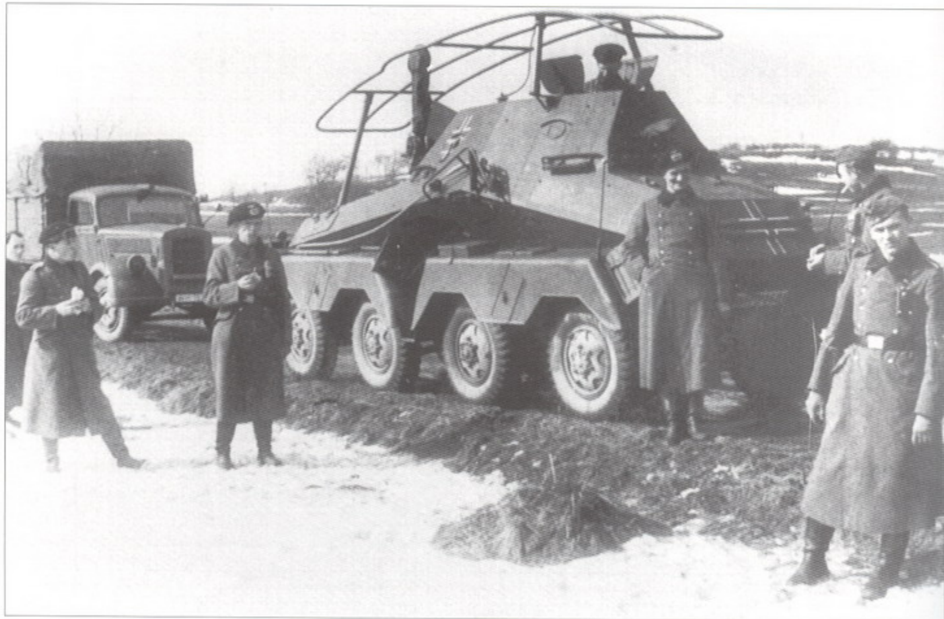
An Sd.Kfz.263 (s.Panzerfunkwagen). Its almost 9-meter telescope antenna mast is folded and covered.
