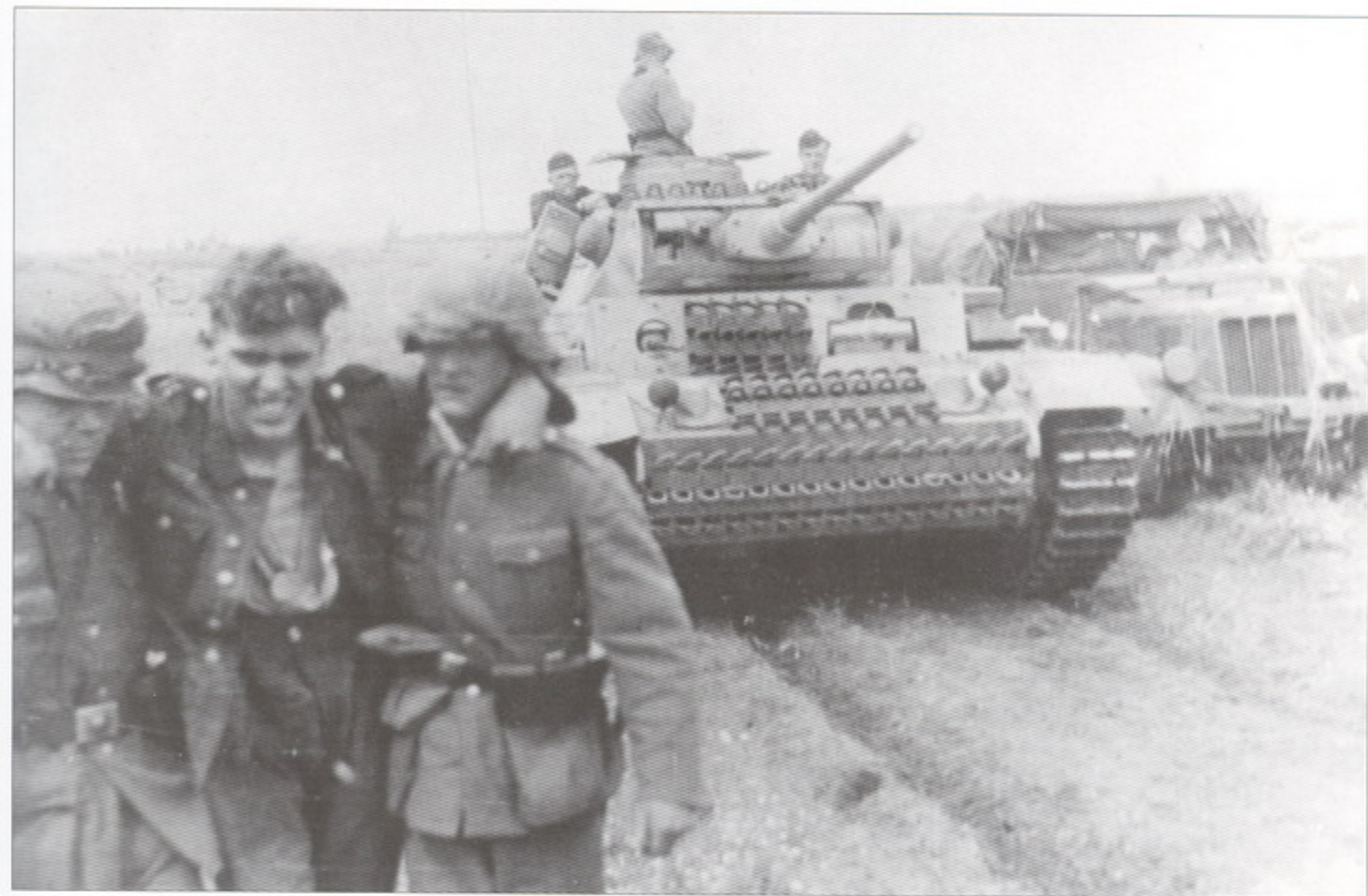
A Pz.Kpfw.III Ausf.L . The often-added extra armor on the gun mantlet was susceptible to damage, and usually only its frame remained after a hit.
