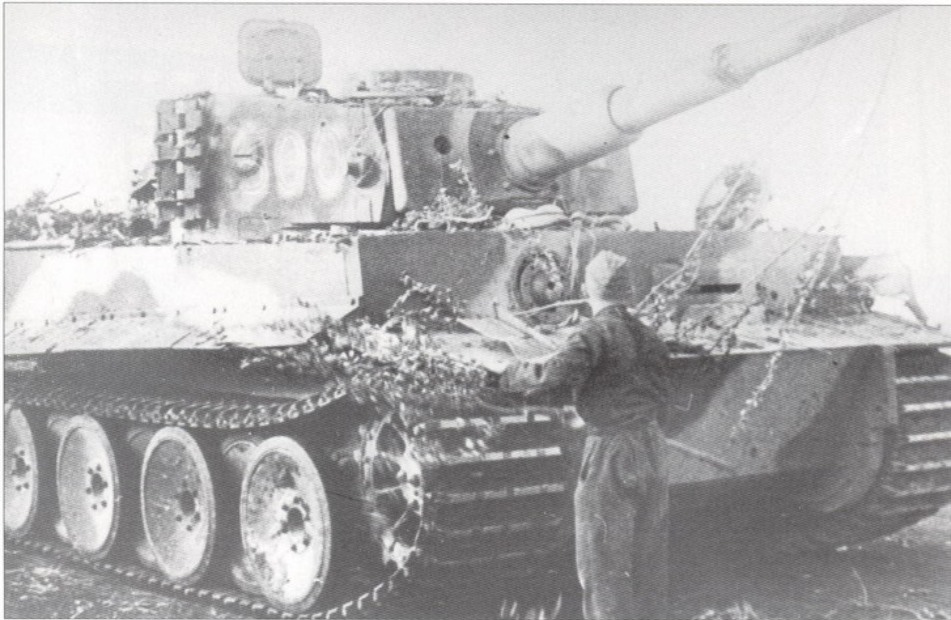
Tiger I with damage to the radio operator's position. The Kugelblende mounting for the machinegun has either been shot off or removed for repairs.
