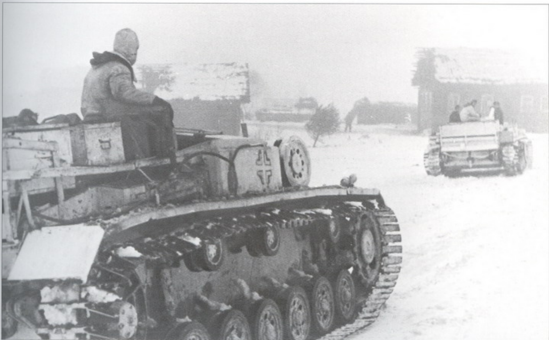
A Sturmgeschütz.III Ausf.E equipped with Ostketten, which improved manoeuvrability during the Russian winter. In the background can be seen a Sturmgeschütz.III Ausf.F , also with Ostketten. Pictured during Operation "Wintersturm" in January 1943, both vehicles belong to Sturmgeschütz.Lehr.Batt. 901 .
