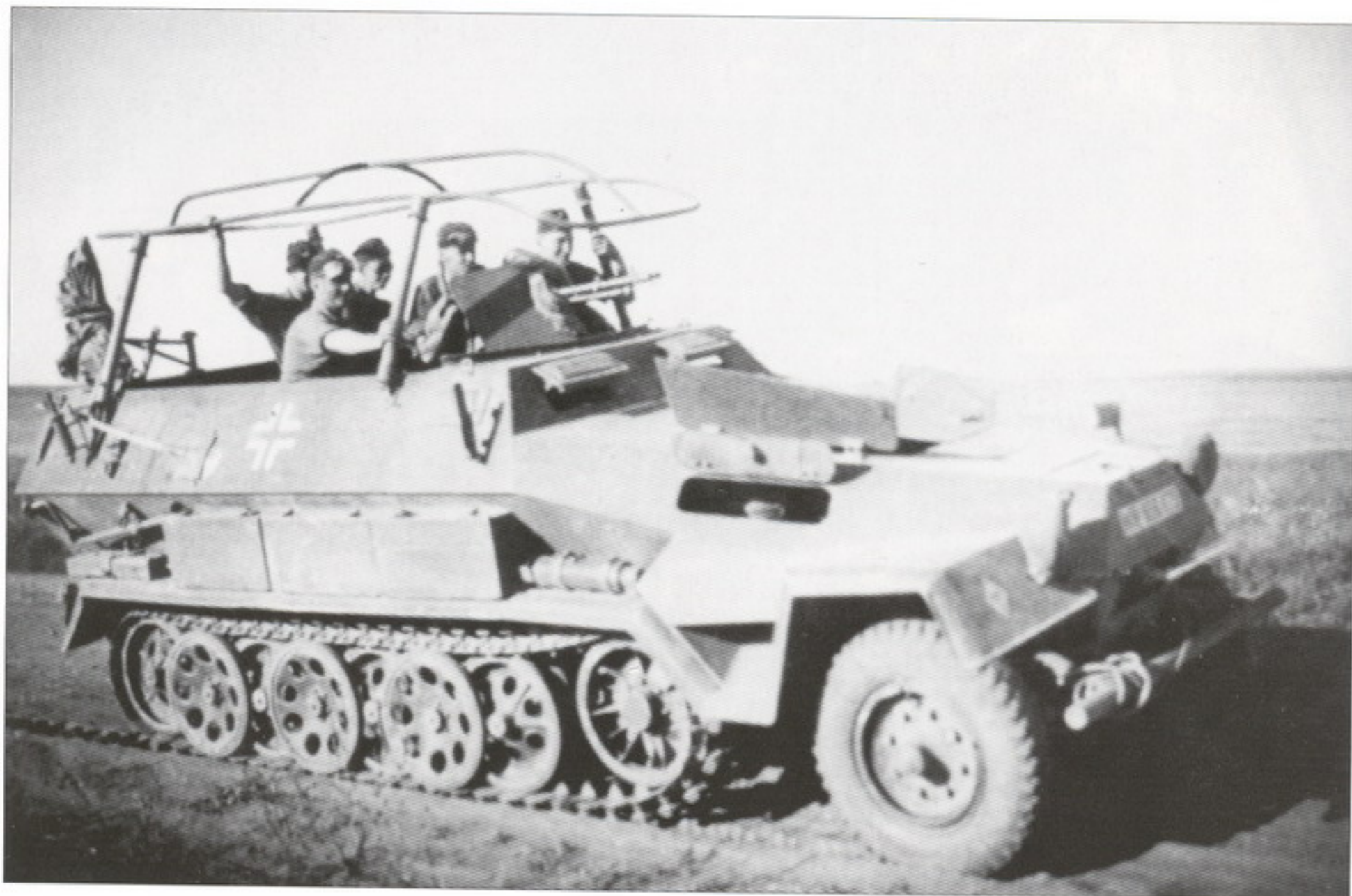
An Sd.Kfz.251/3 Ausf.B (mittlerer Funkpanzerwagen). In the rear part of the vehicle can be seen, covered with tarpaulins, a collapsed FuG. 11 radio mast.
