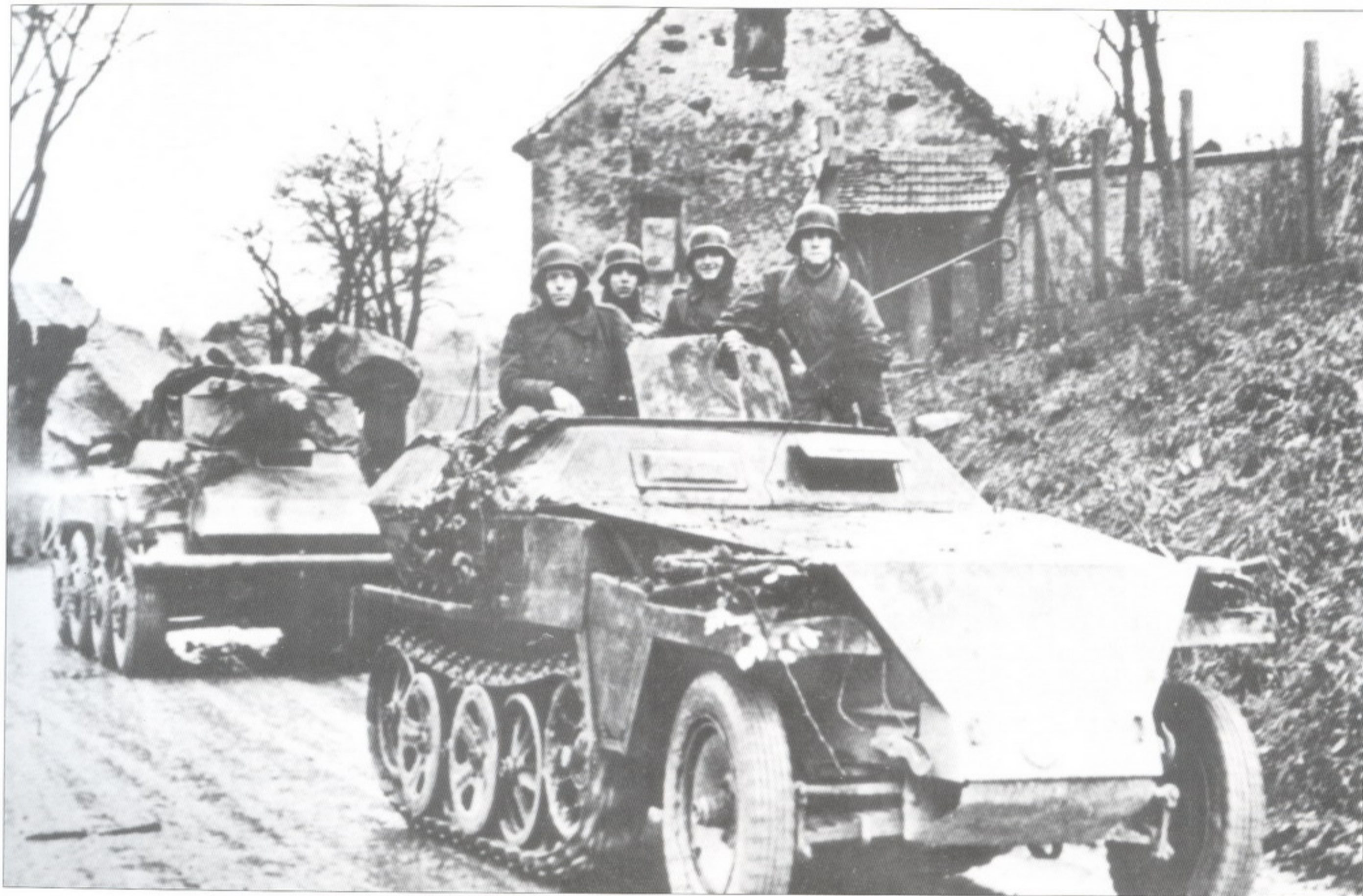
This Sd.Kfz. 250/1 (Neue Ausf.) does not have all of its side containers. In the background can be seen an Sd.Kfz.234/3 (Panzerspähwagen mit 7.5 cm Kanone 51 L/24) . Only 90 vehicles of this type were manufactured.
