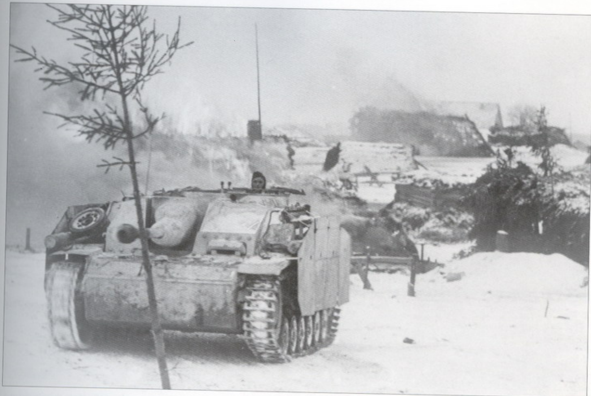
This Sturmgeschütz.III Ausf.G has the Sankopfblende mantlet and the commander's cupola deflector. It is pictured during the battles around Witebsk in February 1944, Army Group Middle.
