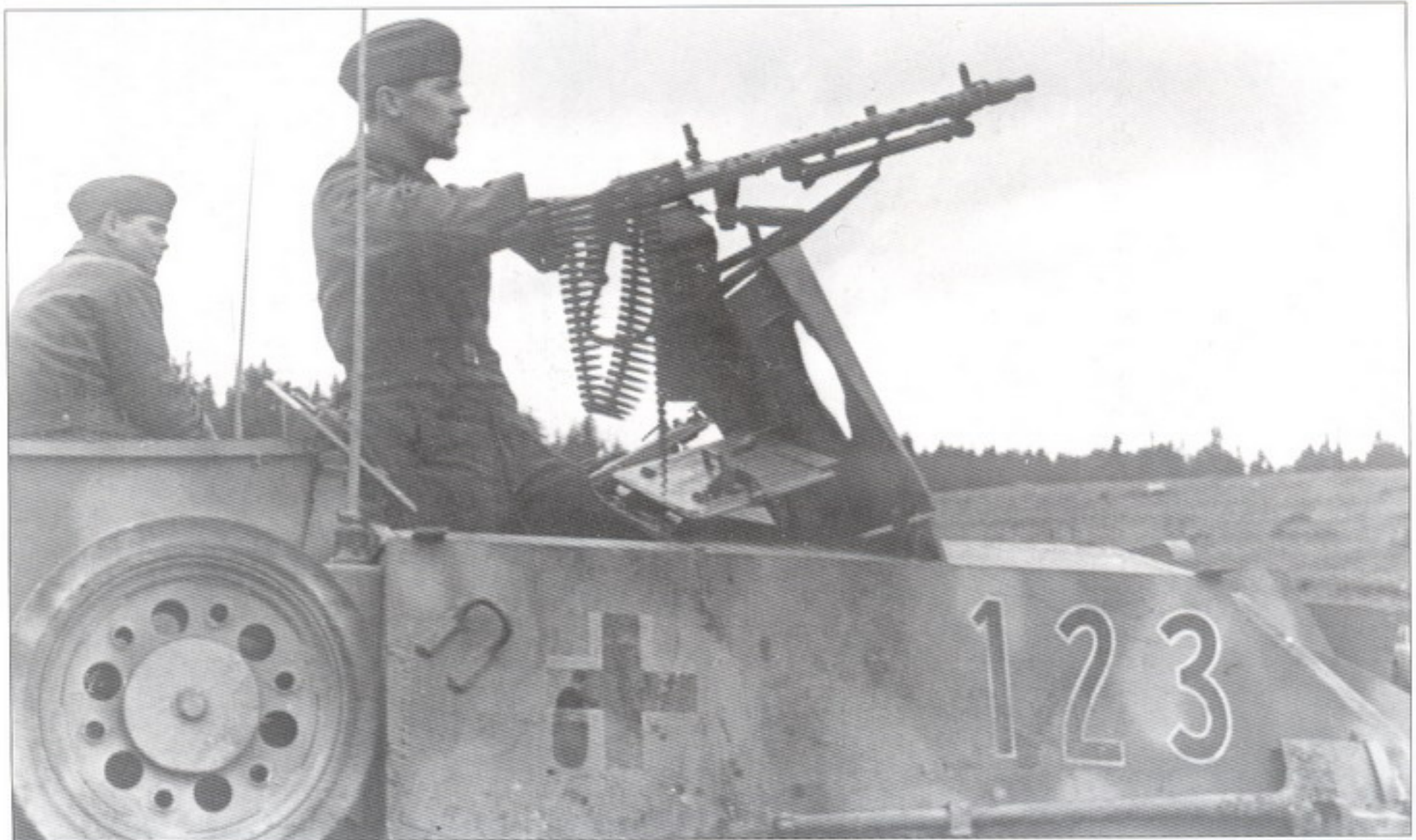
This Sturmgeschütz.III Ausf.G has its machine gun improperly mounted on top of the MG shield, instead of in its slot. While this increased the field of fire, it also increased the danger to the machinegunner as he would forego the protection of the shield.
