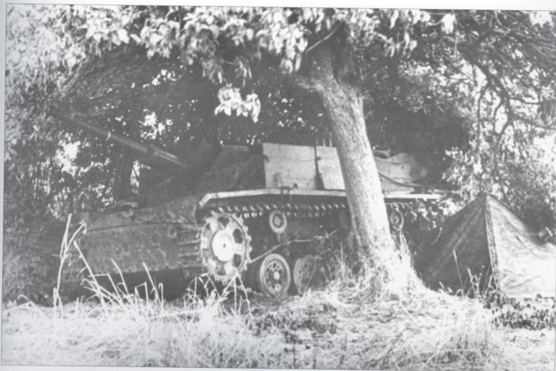
This Sturmgeschütz.III Ausf.G has the added Schürzen. Western Front, August 1944.
