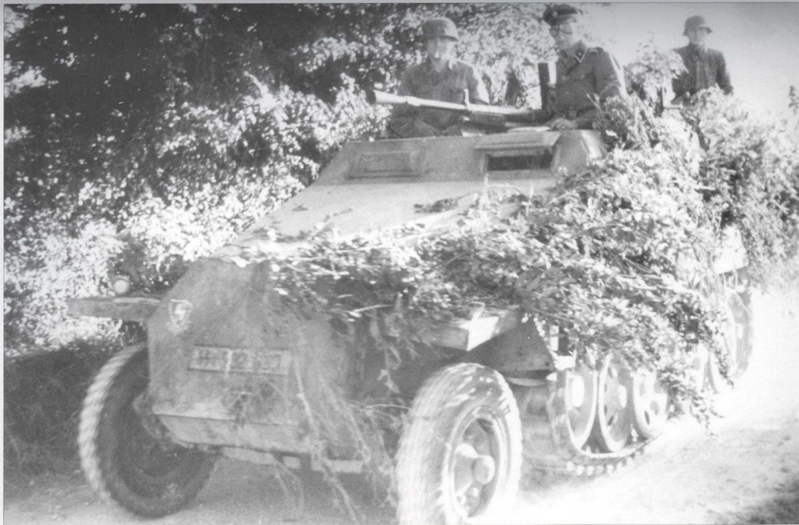
An Sd.Kfz.251/1 Ausf.C of 12.SS Panzer Division "Hitlerjugend" with a field modification, a 2 cm Flak 38. France, summer 1944.
