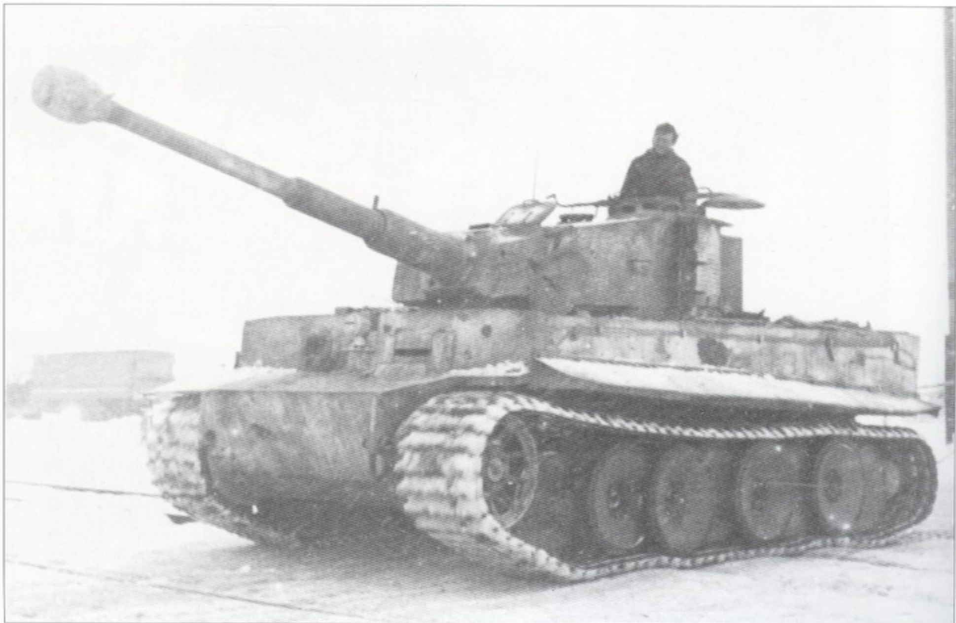
Tiger I sporting well-worn winter camouflage. It has the late-version commander's cupola.
