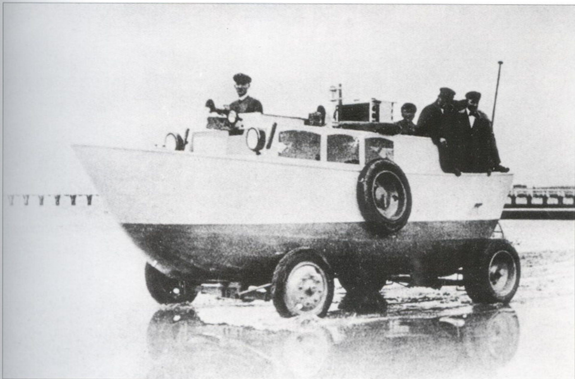
A prototype of an amphibious vehicle from 1929, produced for the Reichsmarine (powered by a 40 HP engine) by the firm of Voran-Automobilwerke in Berlin.
