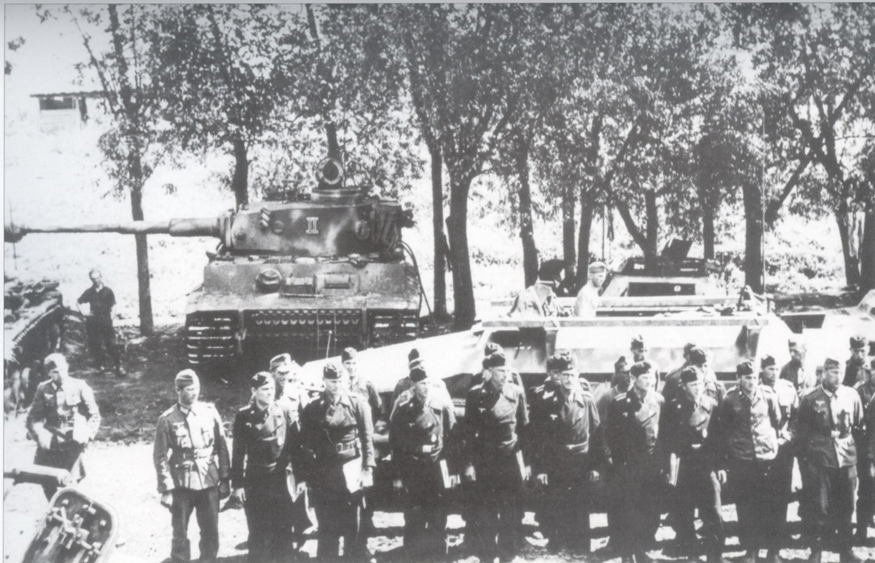
An Sd.Kfz.251/7 Ausf.C (mittlerer Pionierpanzerwagen) with its characteristic brackets for carrying two small engineer bridge spans. In the background is a command Tiger I (Befehlswagen) of s.Pz.Abt.505.
