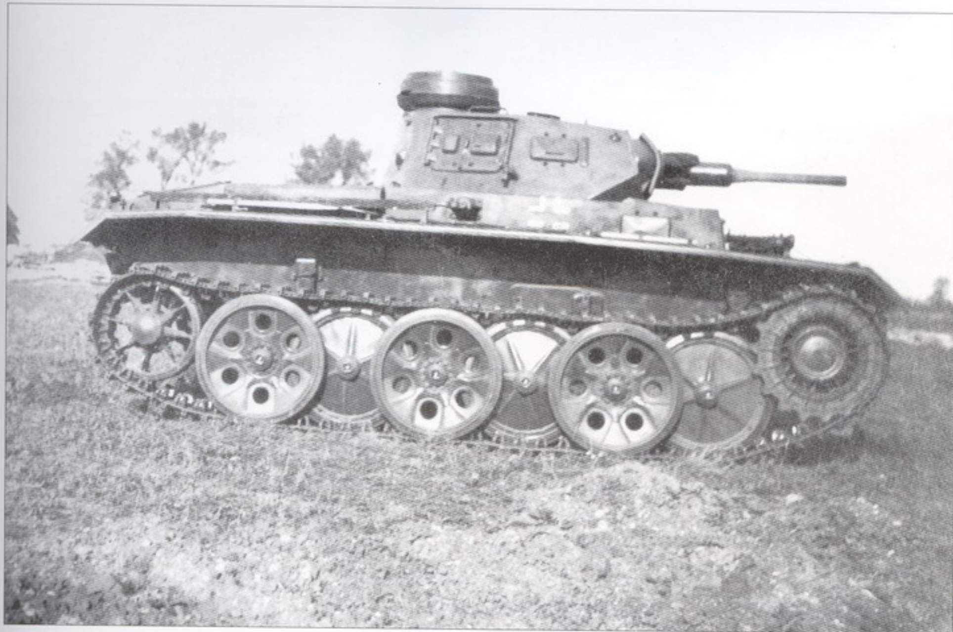
One of the few Pz.Kpfw.III s equipped with the "Schachtellaufwerk" road wheels, supplied by the firm of Famo. This was done under the program of trying to make interchangeable many of the parts of the Pz.Kpfw.III and the Pz.Kpfw.IV .
