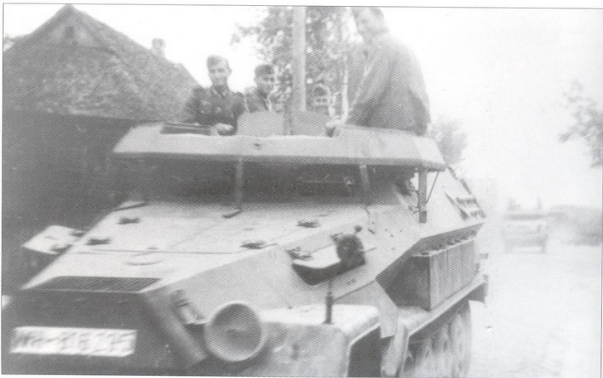
An Sd.Kfz.251/18 Ausf.B of 1.Panzer Division . It has an MG 34 installed and, to improve the field of fire, a portion of the map table has been cut away.
