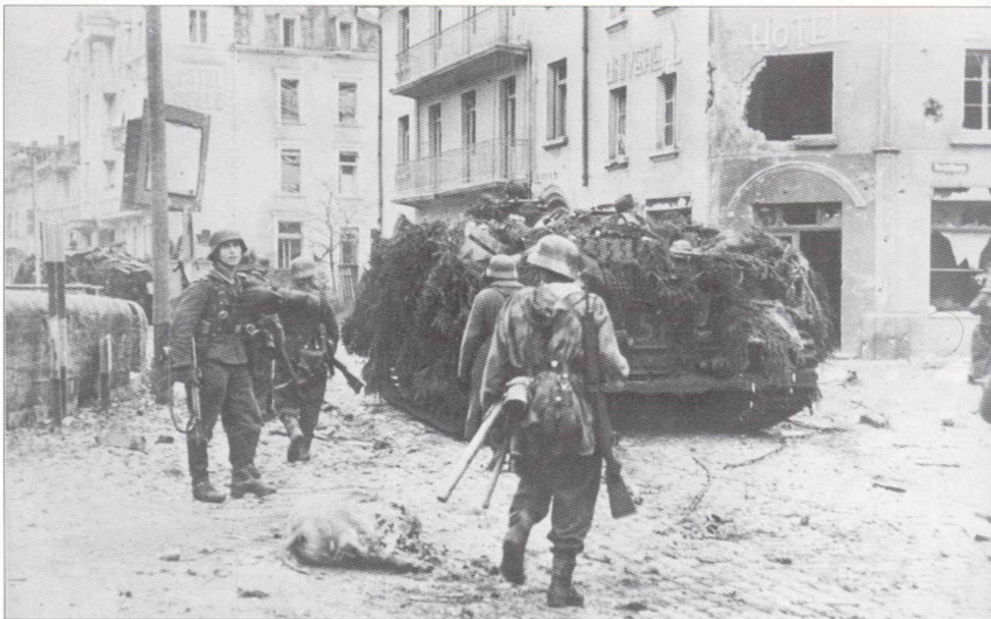
A late production Sturmgeschütz IV with Flammentoter (flame dampeners) on the exhaust pipes. The soldier first from the left has a Sturmgewehr 44 while the others carry the 98 (k) rifle. Western Front, probably October 1944.
