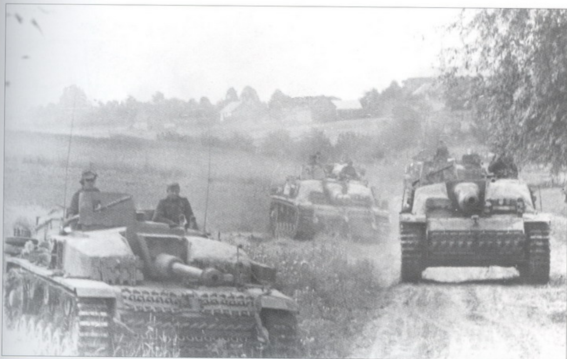
A group of Sturmgeschütz.III Ausf.G sporting the often applied concrete layer on the front of the superstructure. These vehicles probably belong to Sturmgeschütz Brig. 228 which was located on the Eastern Front in August 1944 as part of Army Group South Ukraine.
