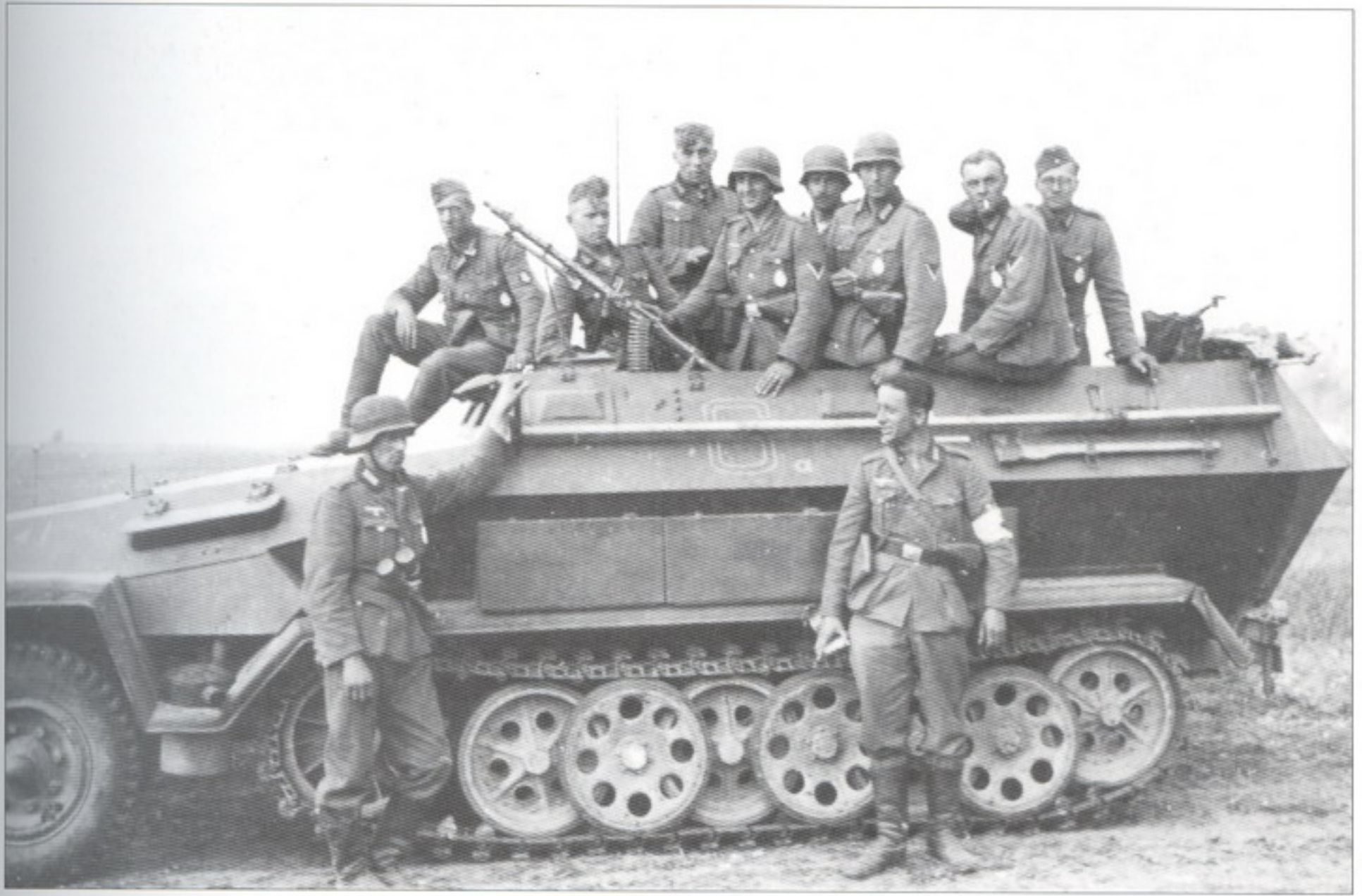
An Sd.Kfz.251/1 Ausf.A , without a gun shield for its forward MG 34. This version had the characteristic 3 vision slits (which could be closed) on the side walls of the superstructure.
