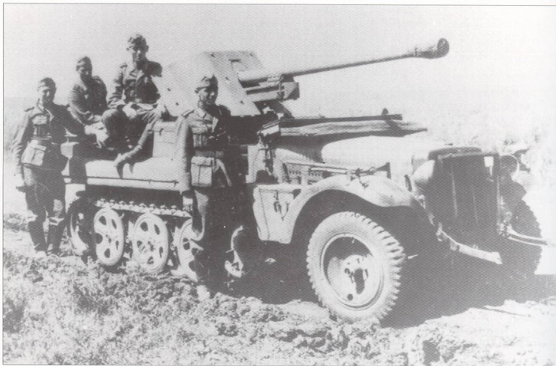
An Sd.Kfz.10 of 13.Pz.Div. with an expedient armament of a 5 cm Pak 38 , Eastern Front, probably 1942.
