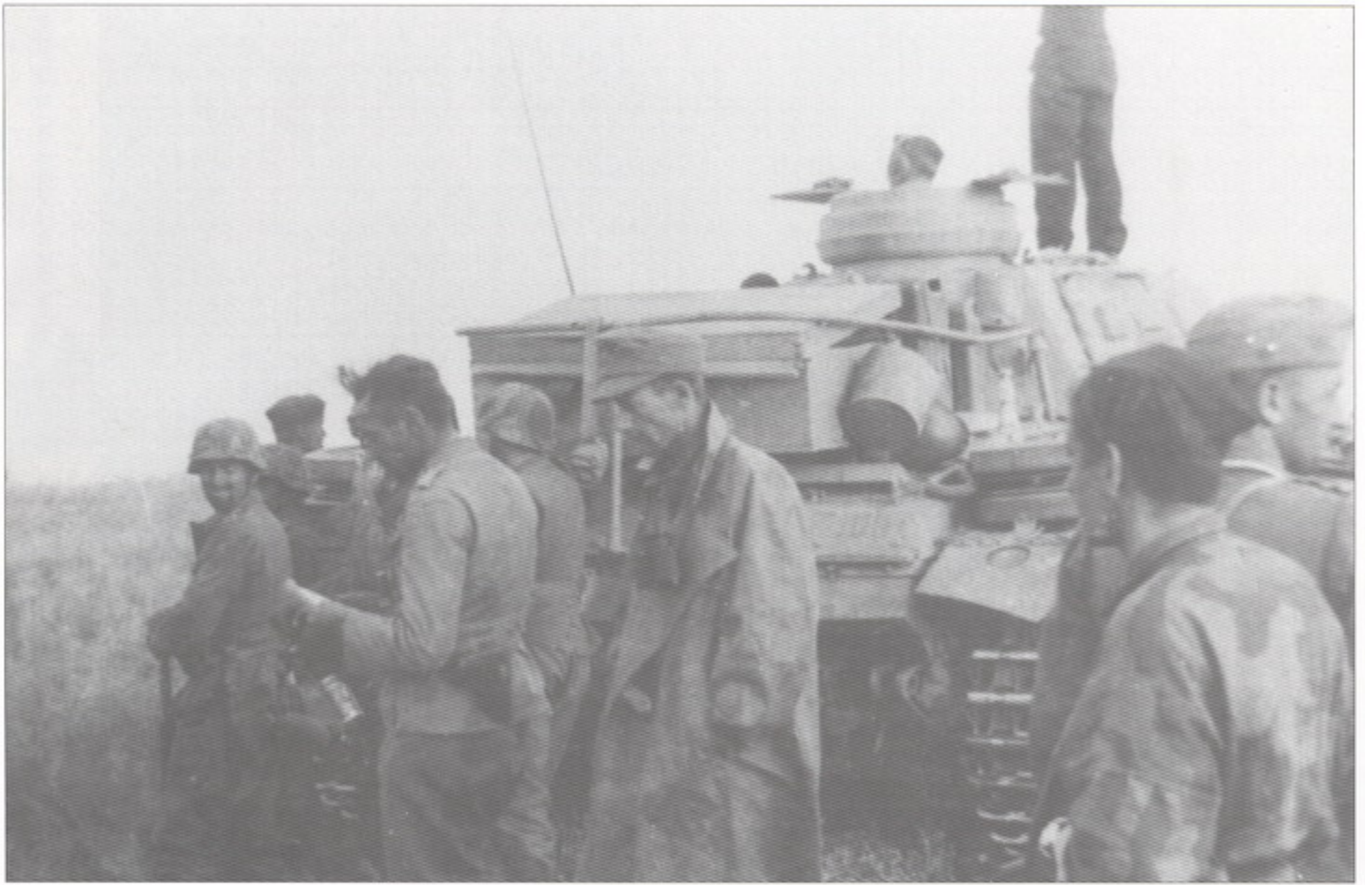
A Pz.Kpfw.III Ausf.H (Befehlswagen) with its characteristic frame antenna installed above the engine compartment.
