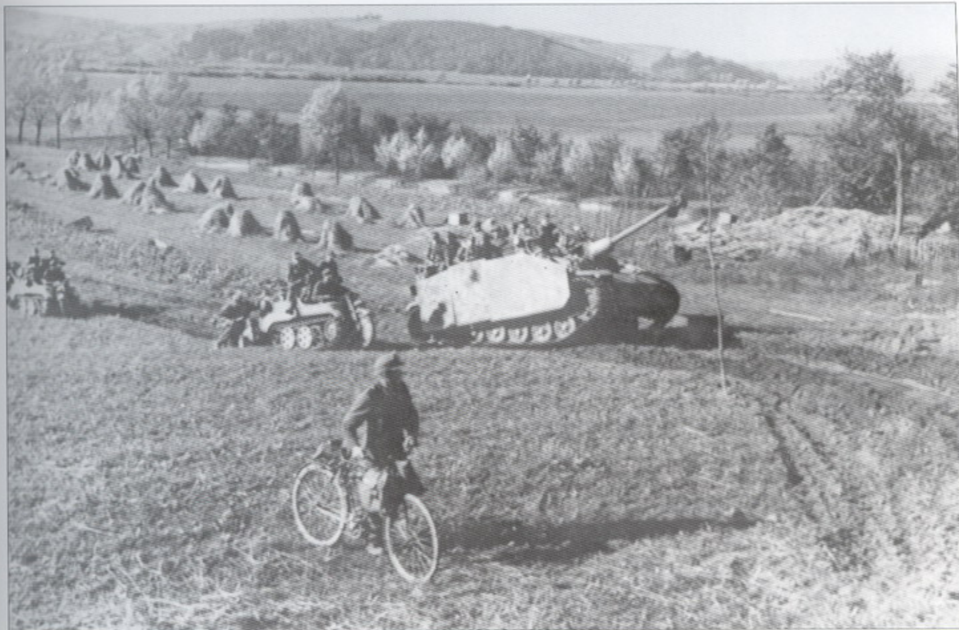
The four-part Schürzen and the Saukopfblende indicate that this is a later series production Sturmgeschütz.III Ausf.G which is leading a column of NSU Kettenrads in 1944.
