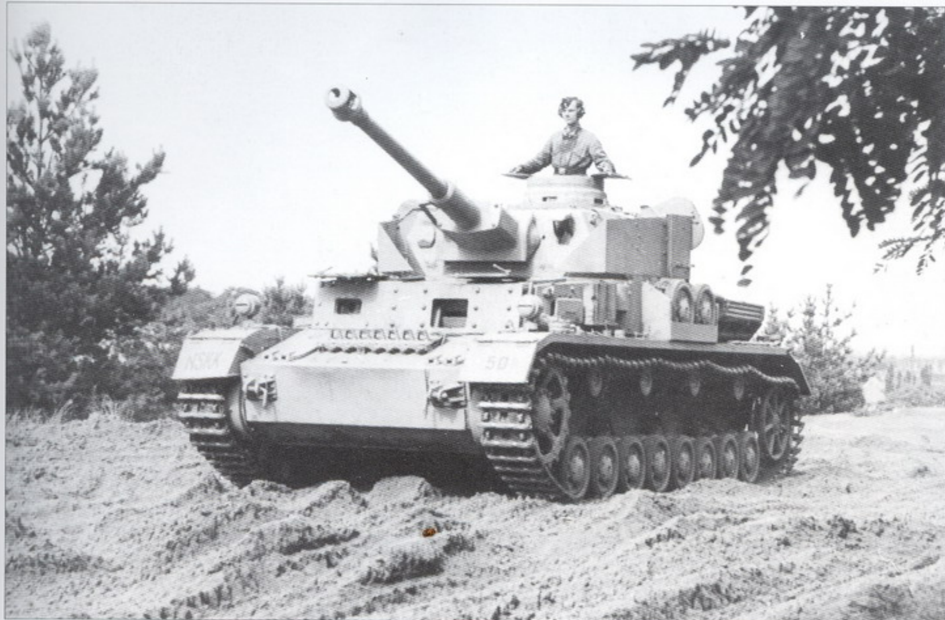
A modified Pz.Kpfw.IV Ausf.D , with a 7.5 cm KwK 40 gun and side Schürzen for the turret.
