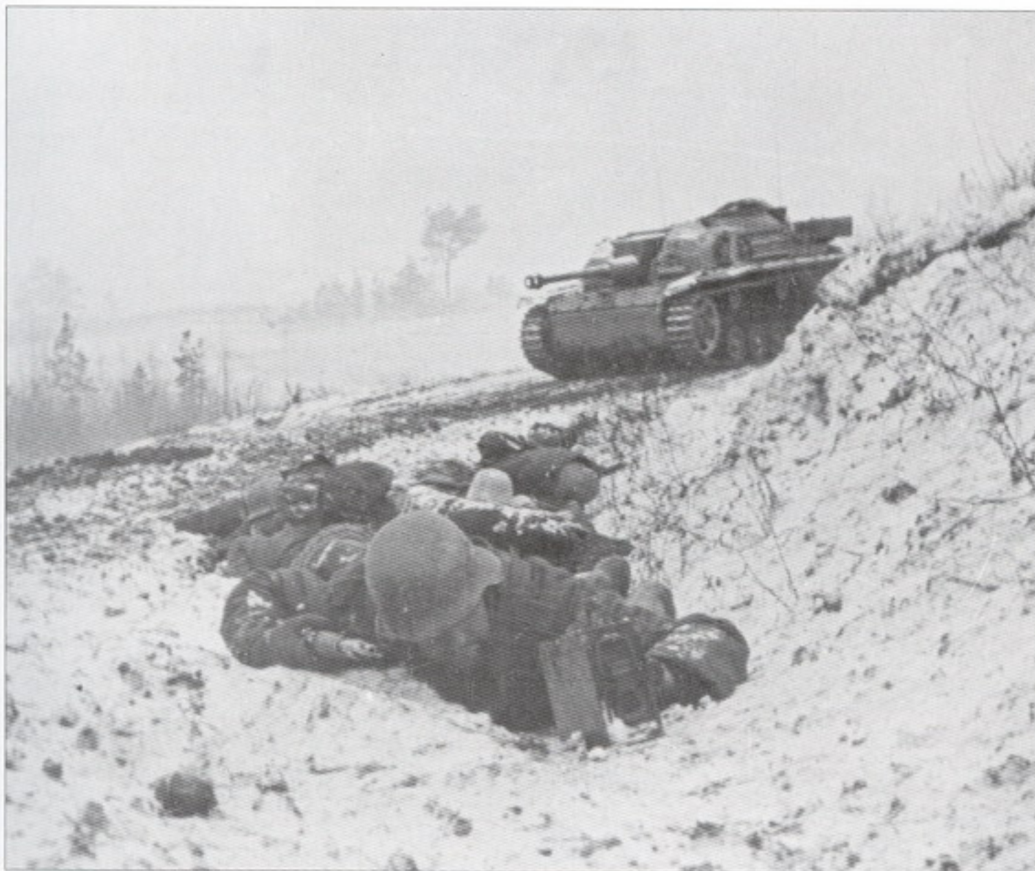
The frontal armor of this Sturmgeschütz.III Ausf.G has been reinforced by a layer of concrete. Ukraine, March 1944.
