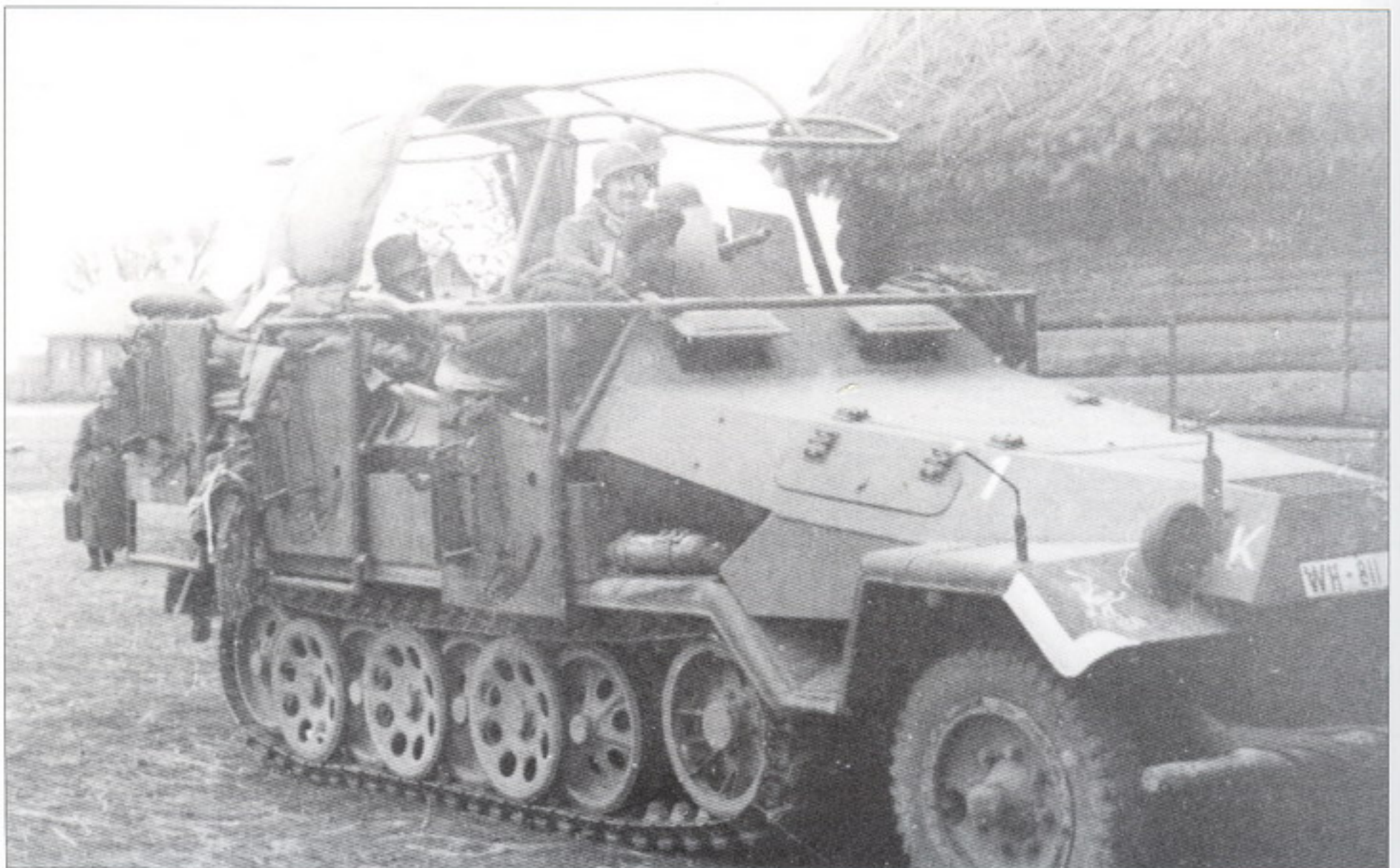
This " Stuka zu Fuss ", an Sd.Kfz.251/3 Ausf.B belonging to 11.Panzer Division , was photographed on the Eastern Front. This is a rare combination of a radio vehicle carrying the Wurfrahmen for the 28 or 32 cm "Wurfgranate" rockets.
